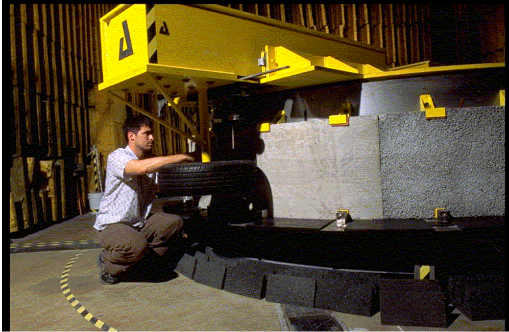
Figure 1. Tire Pavement Test Apparatus (TPTA) located at Purdue University's Herrick Laboratory. (Photo from Purdue University website)
