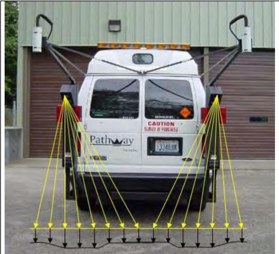
Figure 19. Rut depth measurement using the Pathway Van.
