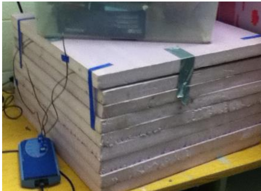
Figure 16. Temperature profile test using top covered, semi-adiabatic test configuration.
