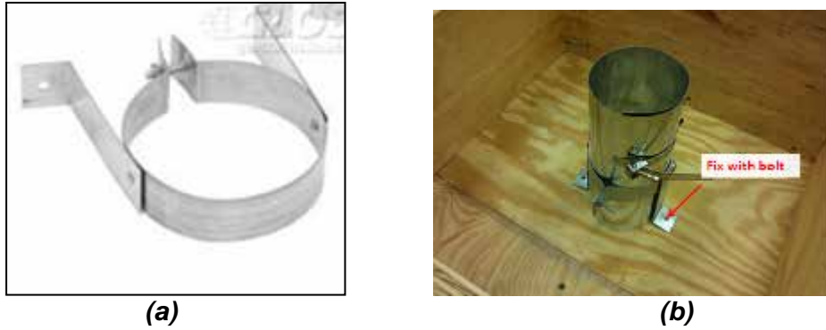
Figure 38. Illustration of in-place cylinder-fastening system: (a) cylinder clamp and (b) form-mounting detail.
