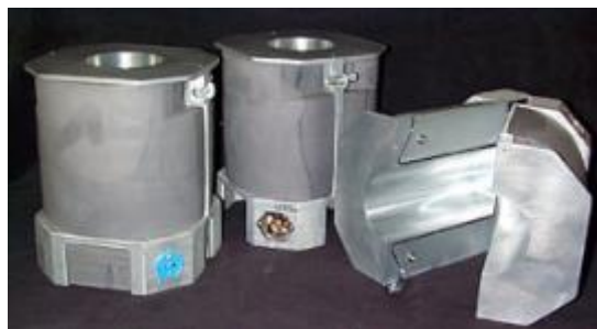
Figure 5. Commercially available equipment for match curing using the insulated jacket molds (TxDOT 2000).
