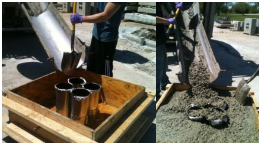
Figure 52. Slab form casting process.
