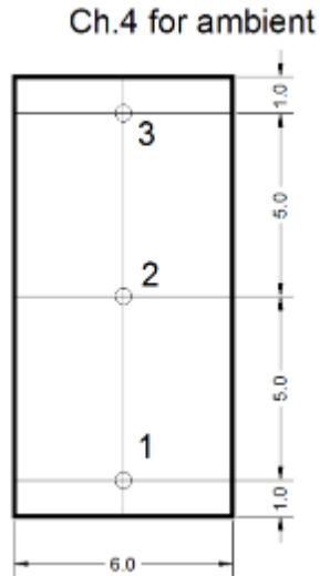
Figure 14. Temperature profile test using semi-adiabatic test configuration: Thermocouple location within cylinder, with dimensions in inches (left) and photo of testing equipment (right). Note: 1 in. = 25.4 mm.
