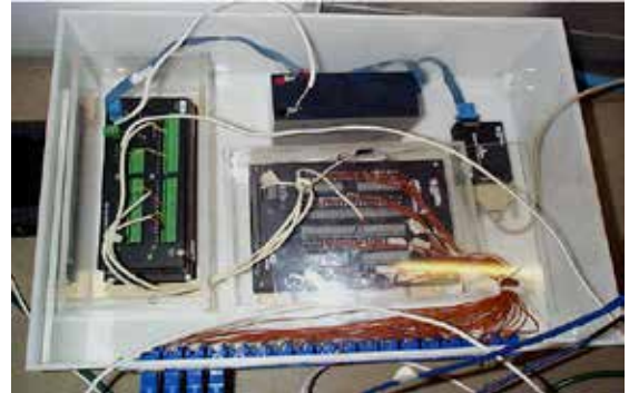
Figure 7. Assembled curing box for air chamber match curing, assembled using off-the-shelf components (Olek 2001).
