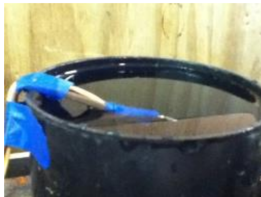
Figure 22. Location of thermocouple in the water-filled 4 x 8-in. cylinder mold.
