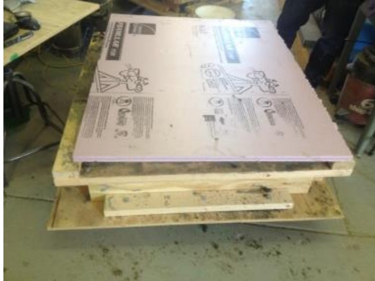
Figure 53. Slab form curing process.
