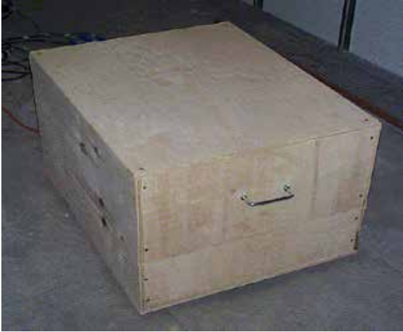
Figure 7. Assembled curing box for air chamber match curing, assembled using off-the-shelf components (Olek 2001).
