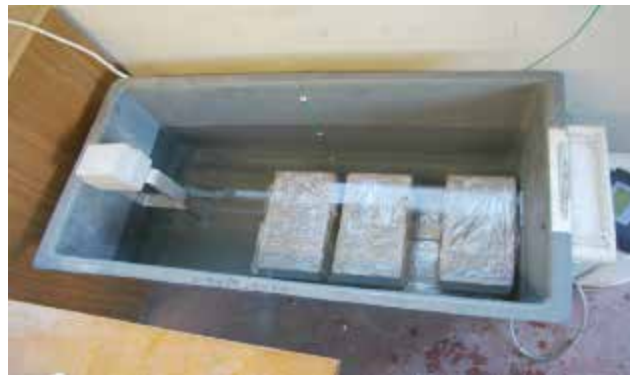
Figure 3. Laboratory equipment for water bath match curing (Reddy 2008).
