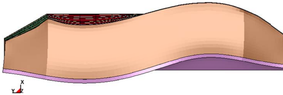
Figure 7-2: Mode shape 2 of the segmental panel wall
