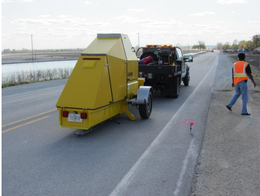
Figure 57. FWD testing on HMA pavement on TS1 (Photo taken on 9/21/11) – Pottawattamie County
