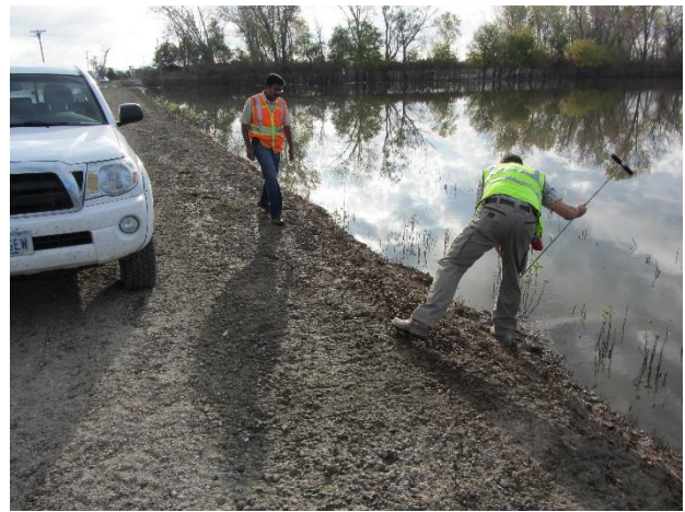
Figure 47. Weep holes detected under a gravel road – Meadowlark Loop Road, Pottawatomie County (Photos taken on 9/22/11)
