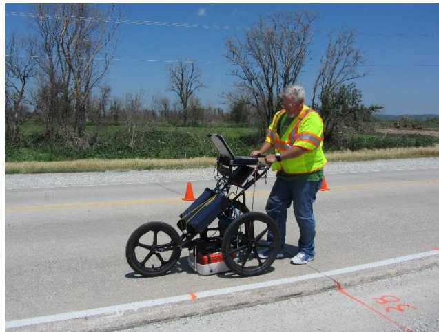
Figure 25. Ground penetrating radar scanning using GSSI SIR-20 data acquisition system
