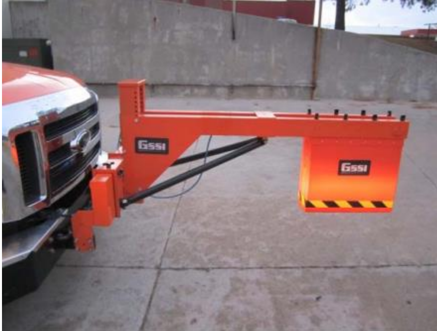
Figure D15. GPR scanning using air-borne (horn) antenna
