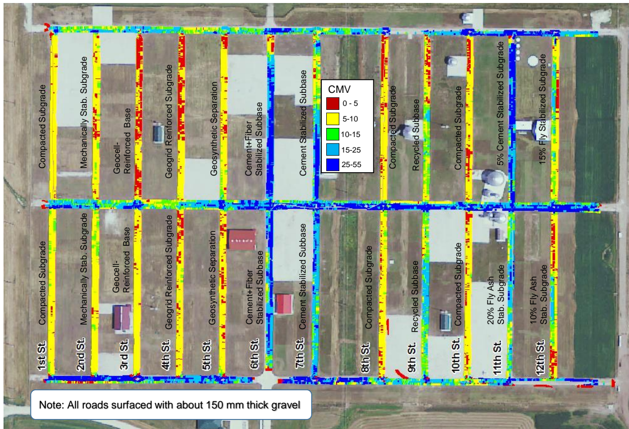
Figure D12. Example RICM spatial map of compaction measurements obtained using CS74 smooth drum vibratory roller after spring-thaw on test sections in Boone constructed using different stabilization methods (White et al. 2013b)
