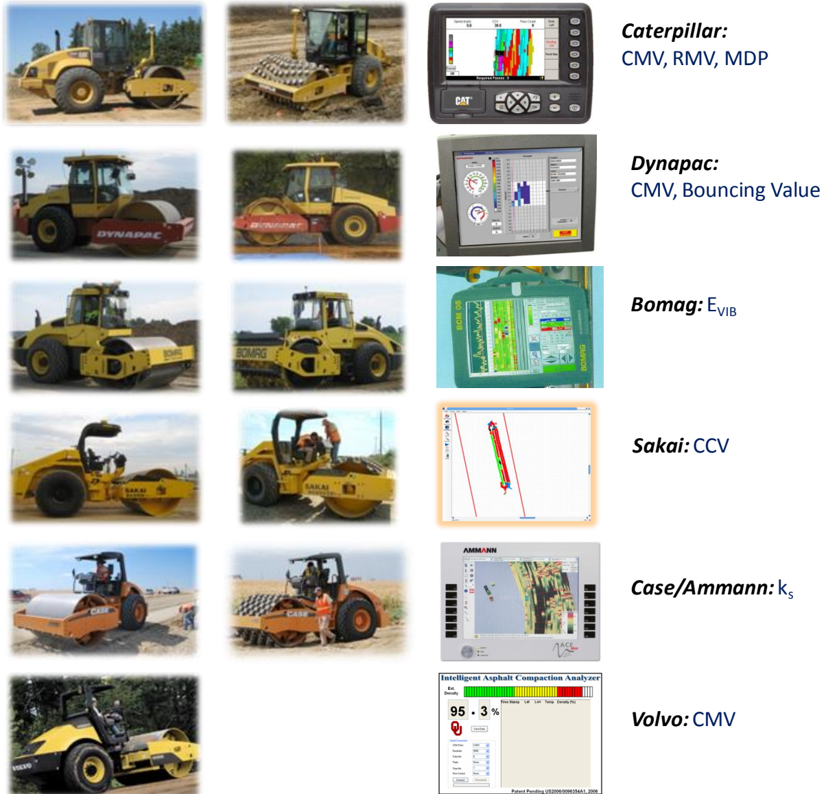
Figure D11. Pictures of various roller manufacturers, roller configurations, and display software's with RICM technology (note that this does not represent a complete list)
