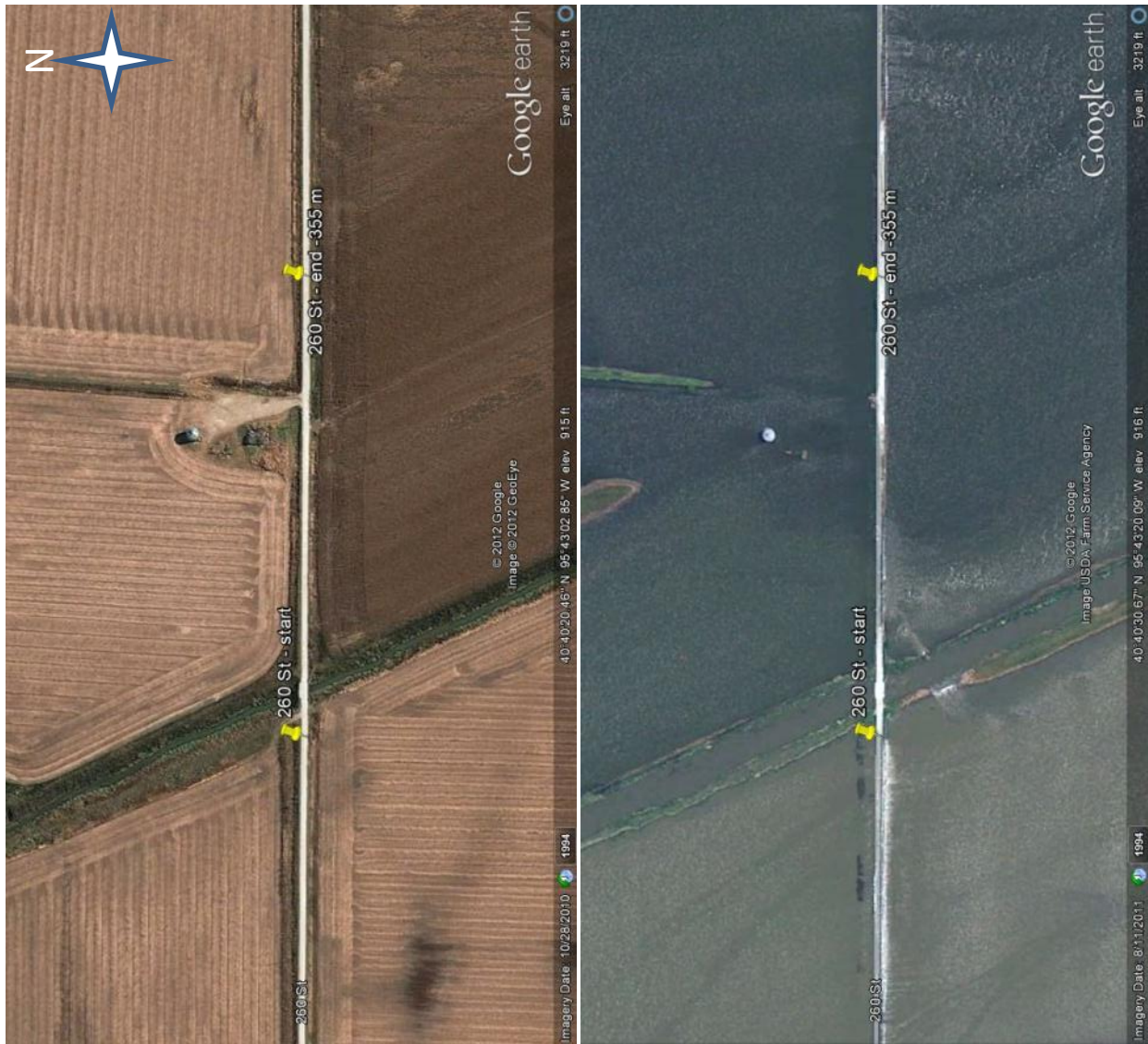
Figure 129. Aerial imagery before flooding on left (from 10/28/10) and during flooding on right (from 8/11/11) on TS1 – Fremont County
