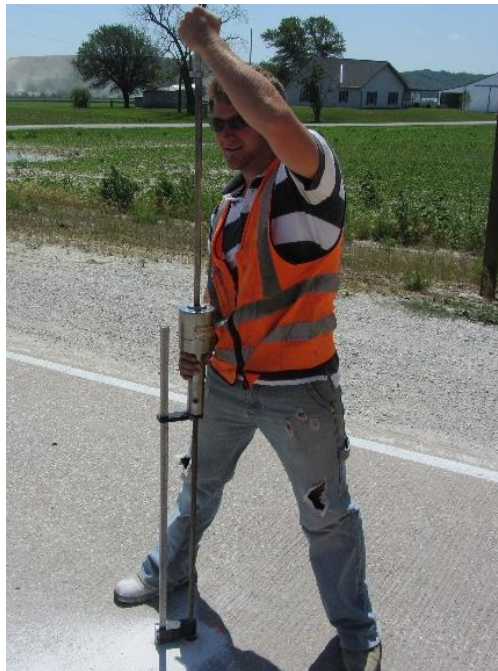
Figure 17. Dynamic cone penetrometer (DCP)
