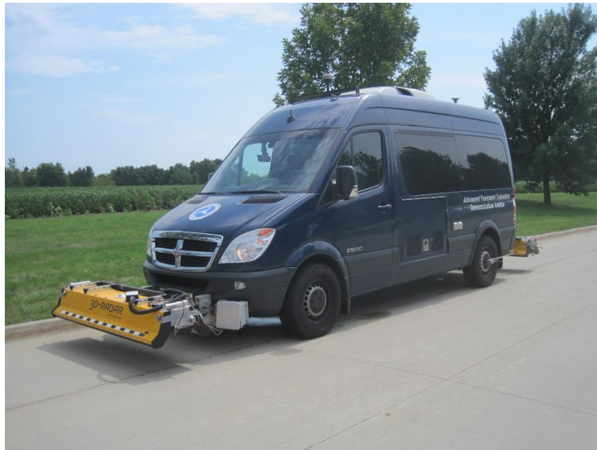
Figure D16. FHWA step-frequency GPR (Courtesy of Jim Grove, FHWA)
