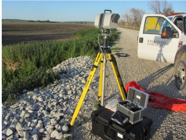
Figure 26. Trimble CX 3D laser scanner
