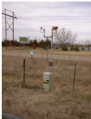
Figure 12. Photo. Mini site-specific SMP weather station used to record climatic data.
