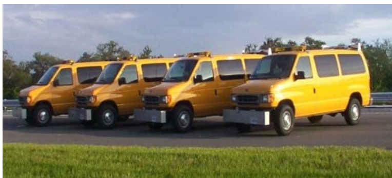
Figure 7. Photo. Inertial road profilers used to measure IRI, RN, and other roughness indices.
