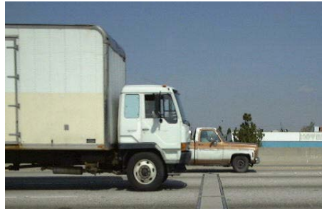
Figure 11. Photo. WIM sensor used to record truck axle and gross vehicle weights.
