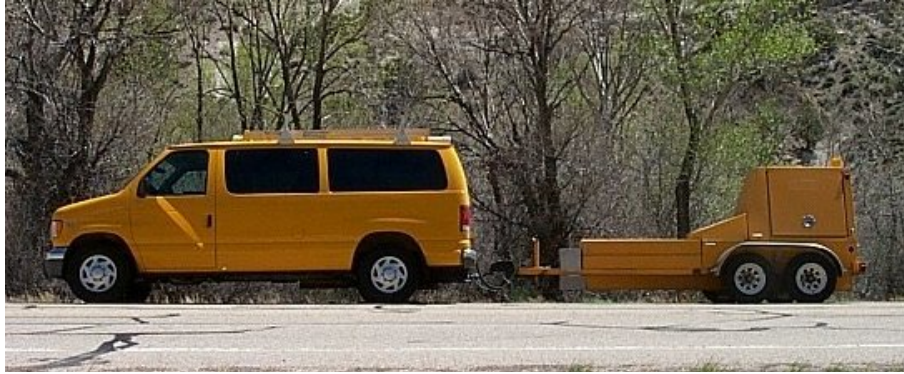
Figure 8. Photo. FWD used for structural evaluation.
