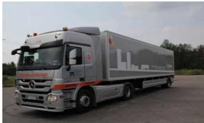
Figure 9. Photo. TSD used for structural evaluation.
