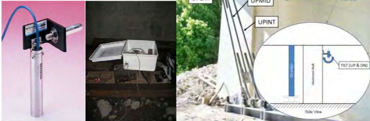
Figure 7.4: Tilt Meter on Abutment Wall, USG Bridge (UCII, 2012)
