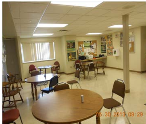
Figure 4.24. Example of instances where unnecessary lighting was being used in unoccupied areas
