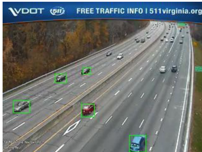
Figure 5. Detected vehicles under good conditions — realistic video 1, example frame 1
