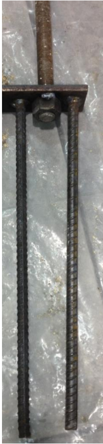
Figure 5.16: Deep T-girder specimen with anchor bars welded to the washer plate
