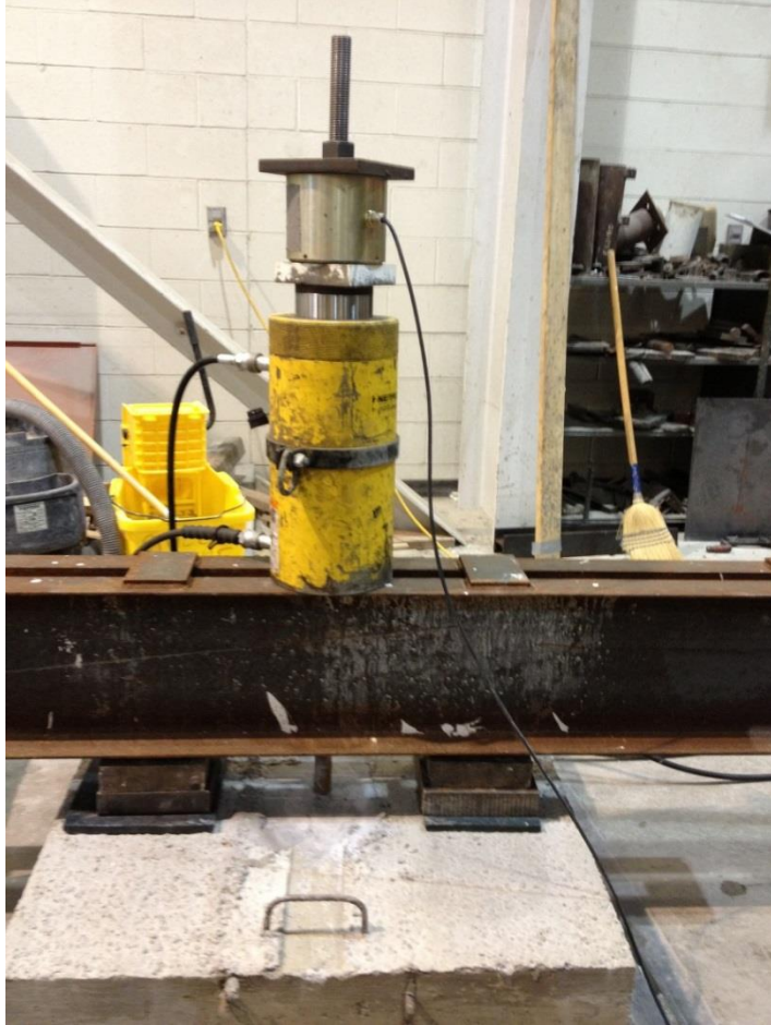
Figure 5.23: Pullout test setup
