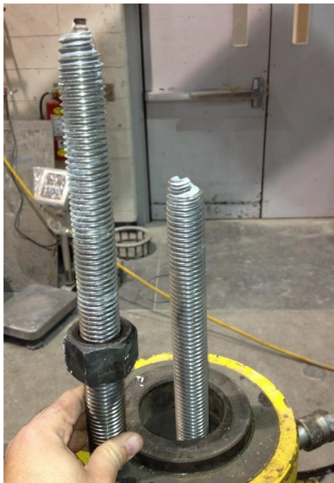
Figure 5.17: Rupture of the TR
