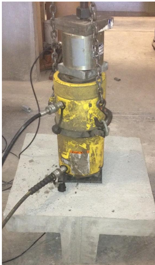
Figure 5.8: Pullout test setup of shallow T-girder specimens
