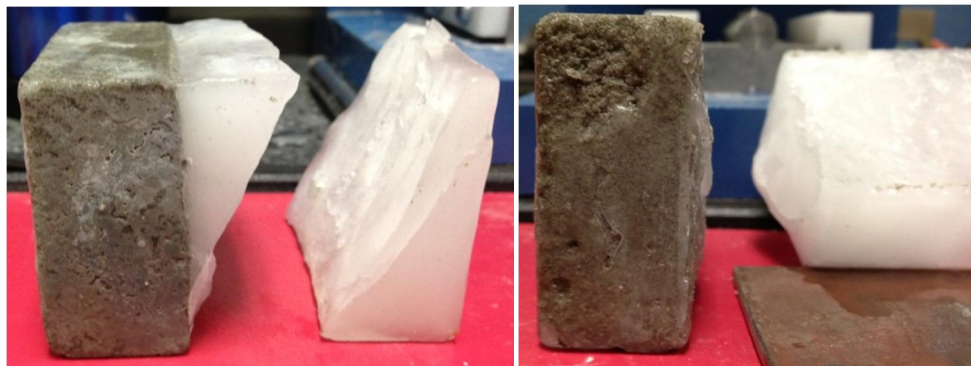
Figure 23: The ice fracture patterns of uncoated (left) and coated (right) specimens
