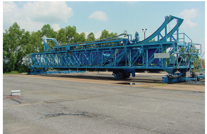
LTRC’s Accelerated Loading Facility
