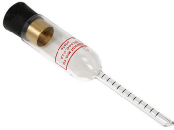
Figure 4.4 Air indicator and brass cylinder tube used for measurement of air content.
