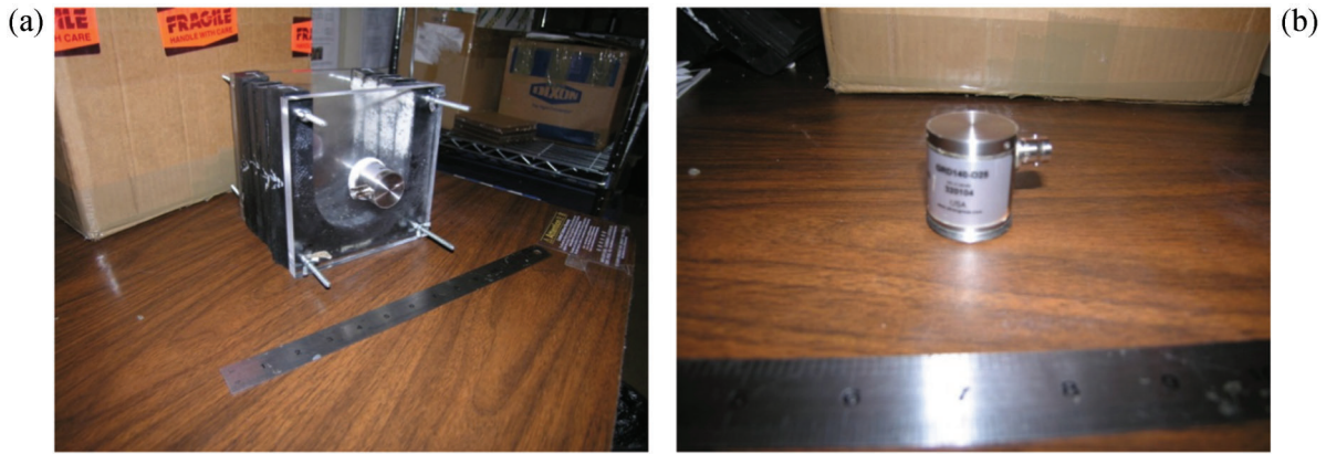
Figure 2.4 (a) Revised test rig with rubber wall. (b) Ultrasonic transducer.
