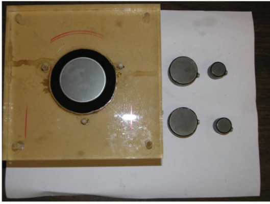
Figure 2.6 Ultrasonic transducers used in present study: 1-MHz transducer (right), 500-kHz transducer (center), and 100-kHz transducer (left).
