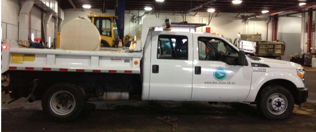
Figure 4.12: The 130 Gallon Tank on One Ton Truck used for Herbicide Spraying prior to Epoke.
