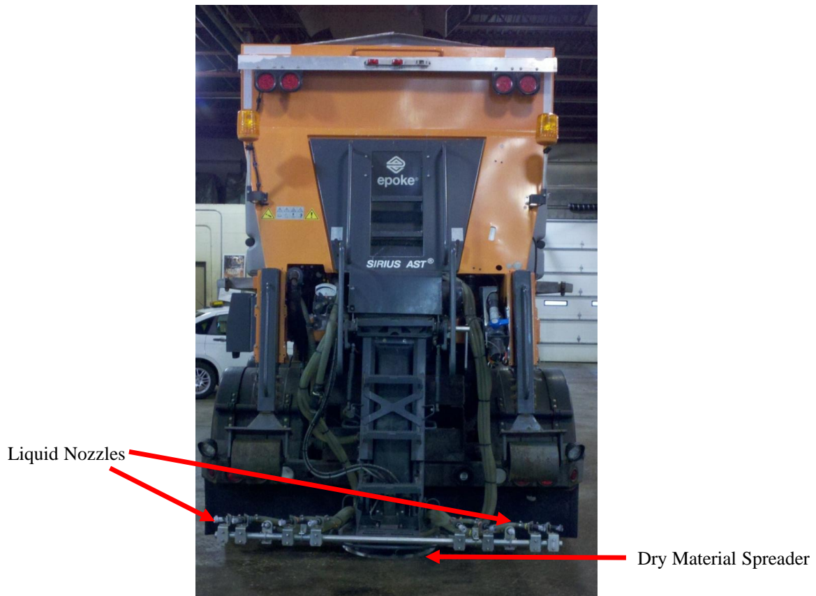
Figure 3.7: Dry Material Spreader and Liquid Nozzles on the Epoke.
