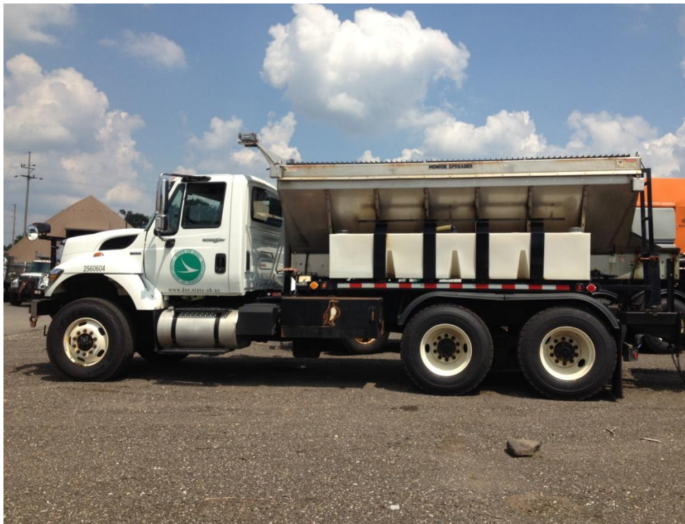
Figure 3.3: Standard ODOT Spreader on Tandem Axle Dump Truck.
