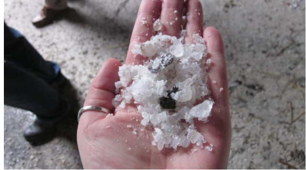
Figure 3.5: Salt Consistency after Crushing by Epoke and Standard Salt.
