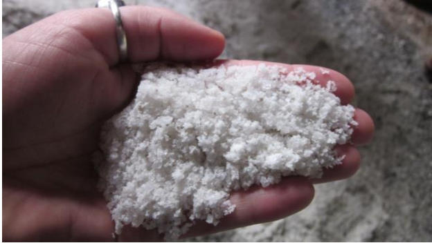
Figure 3.5: Salt Consistency after Crushing by Epoke and Standard Salt.
