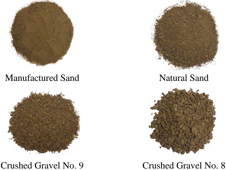
Figure 3.3: Picture of Aggregates Used to Prepare Crushed Gravel Aggregate Blend.
