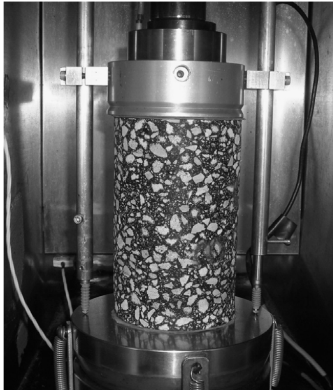
Figure 4.8: Attachment of LVDTs for Flow Number (FN) Testing.
