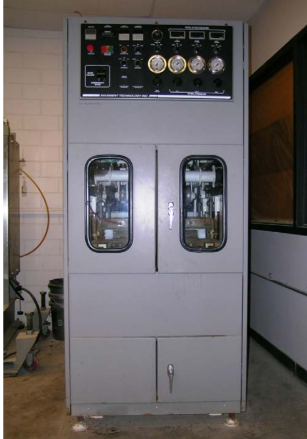
Figure 4.2: Asphalt Pavement Analyzer (APA).
