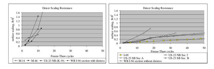
(a) (b) Figure 3.10 Laboratory deicer scaling results for field concrete projects with (a) and without (b) joint associated distress
