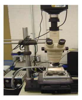
Figure 2.4 Digital microscope setup.
