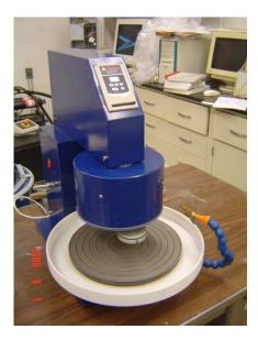
Figure 2.5 Concrete polisher (www.concrete-experts.com)
