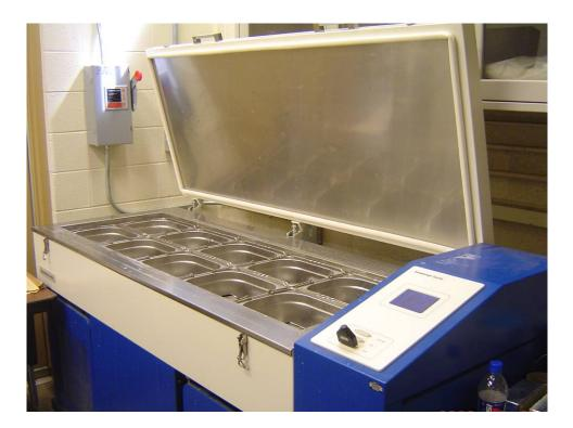
Figure 2.2 Freeze-Thaw Machine (www.schleibinger.com)
