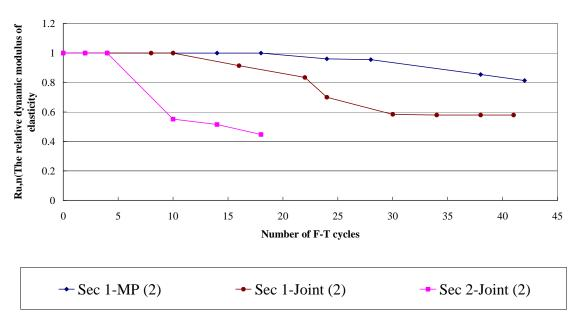
I-94 : Evaluation of the internal damage: Water
