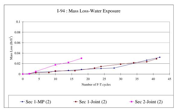
Figure A-13 Mass-loss due to combined freeze-thaw and water exposure
