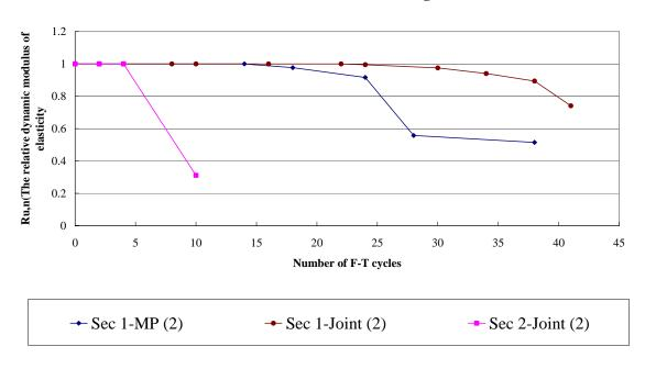
I-94 : Evaluation of the internal damage: De-icer
