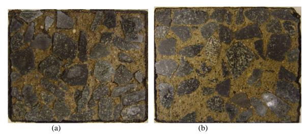
Figure 3.17 Control concrete with 7.3 % air (a), and slag-cement concrete with 5.8 % air after 42 freezethaw cycles in salt solution
