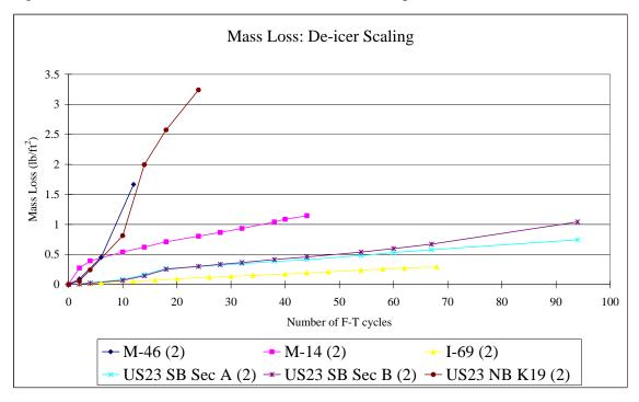
Figure A-6 Mass-loss due to freeze-thaw and deicer salt exposure
