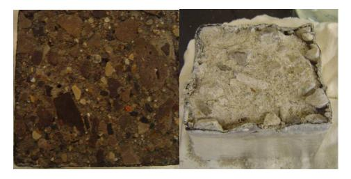
(a) (b) Figure 3.9 Concrete exposure surface from WB I-94, Lawrence, without associated joint distress (a) after 12 freeze-thaw cycles, and (b) from the distressed area after 10 freeze-thaw cycles.
