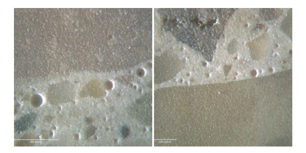
Figure 3.1 Typical interface zone in slag cement concrete
