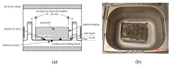
Figure 2.3 Close-up of specimen test (a) and actual test specimen with bottom test surface in contact with liquid, in this case in a frozen condition (b).
