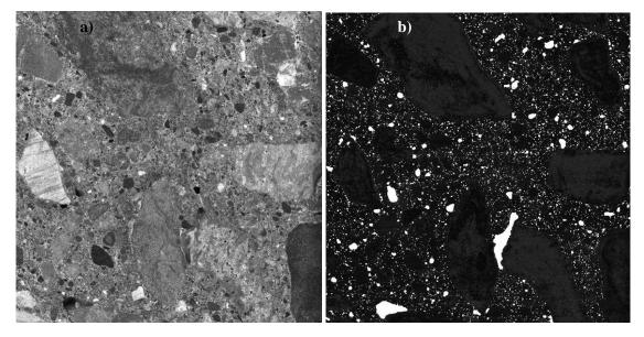
Figure 2.6 Sample surface after polishing (a), and the same surface after contrast enhancement (b).
