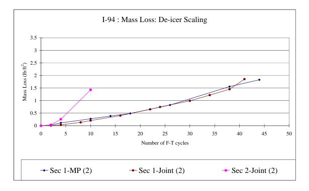
Figure A-14 Mass-loss due to combined freeze-thaw and deicer salt exposure
