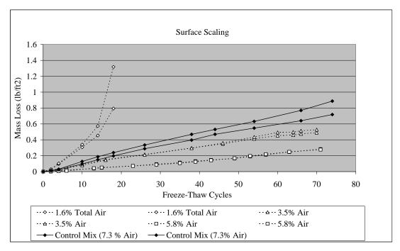
Figure 3.15 Mass loss of various air content concrete in de-icing solution
