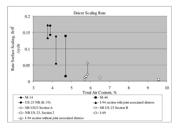
Figure 3.11 Deicer scaling rate for field concrete versus air content.
