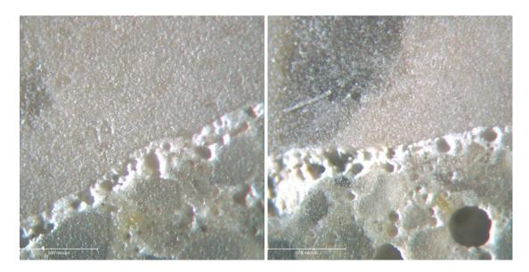
Figure 3.19 Highly porous interface zone (agglomeration of air-voids) around the coarse aggregate in the control concrete.
