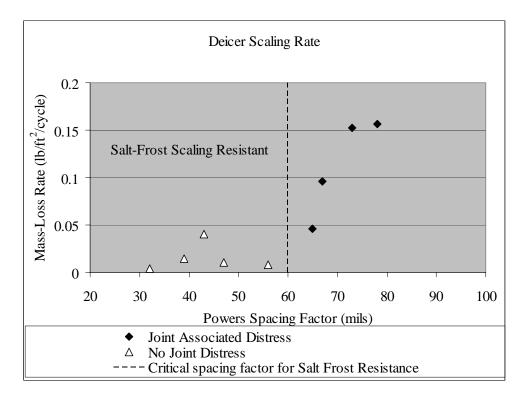
Figure 3.13 Deicer scaling rate versus Powers Spacing Factor
