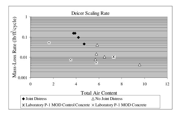
Figure 3.16 Scaling rate for P-1 MOD lab concrete and field concrete
