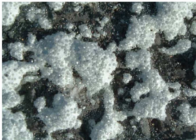
Figure 40. Photo. Glass beads in MMA.
