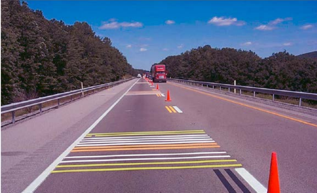
Figure 1. Photo. Example of NTPEP removable tape transverse test deck.
