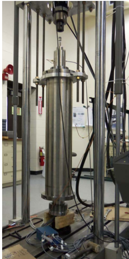
Figure 4-12 The test vessel rated for a pressure of 34 MPa
