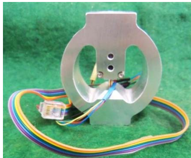
Figure 4-11 Proving ring with 44.5 kN capacity that was used to validate the loading of the chain of specimens
