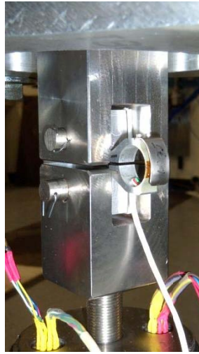
Figure 5-1 Image of specimen pre-fatiguing. A CMOD gage is shown inserted at the load line. The specimen is connected to the clevises via pins.
