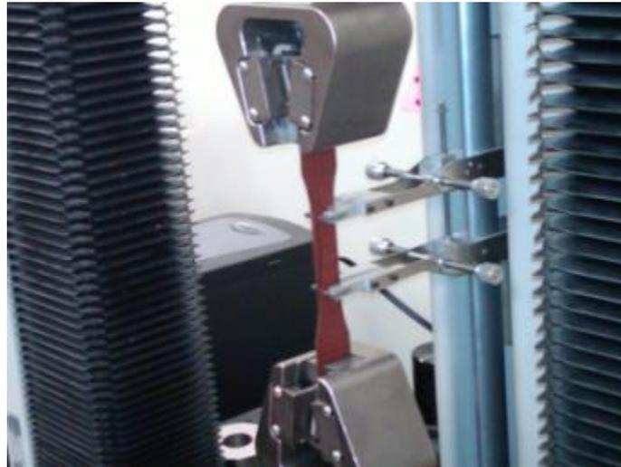
*Figure 14 - ASTM D3039 tensile test specimen*
