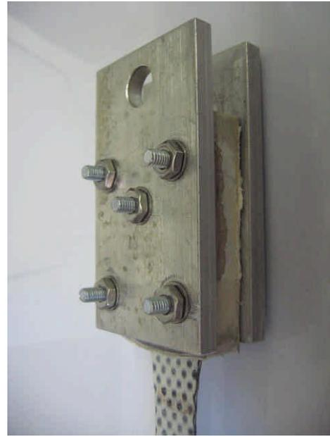
**Figures 11 & 12. Epoxy Block and Plate Clamp for Carbon Creep Tests**
