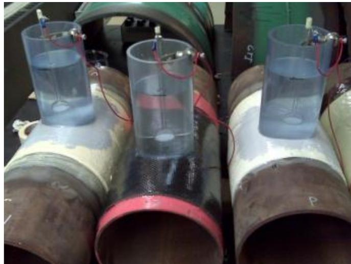
*Figure 45 - Installation of the test cells on the composite samples*
