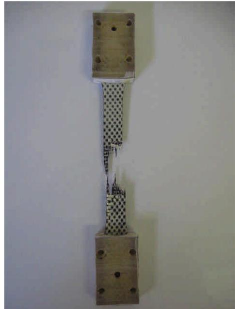
**Figures 9 & 10. Creep Ruptures for Fiberglass and Carbon at 60% UTS**
