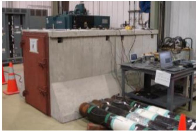
*(b) The pressure test chamber and equipment*
