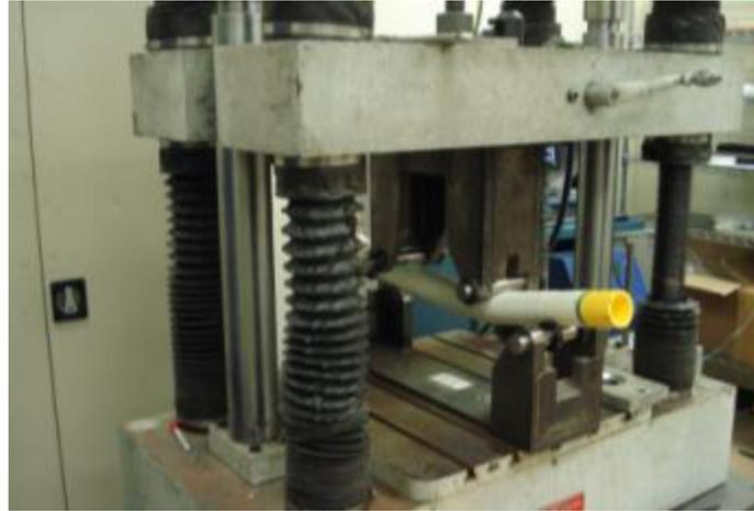
*Figure 32 - Composite sample under four-point loading test*
