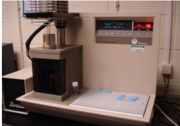
Figure 55 - The thermo-mechanical analyzer
