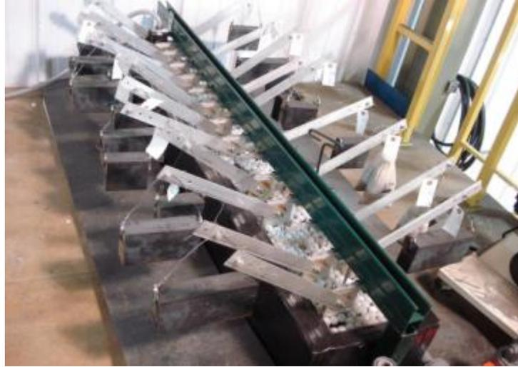
*Figure 22 - View of the loading frames in temperature-controlled containers*
