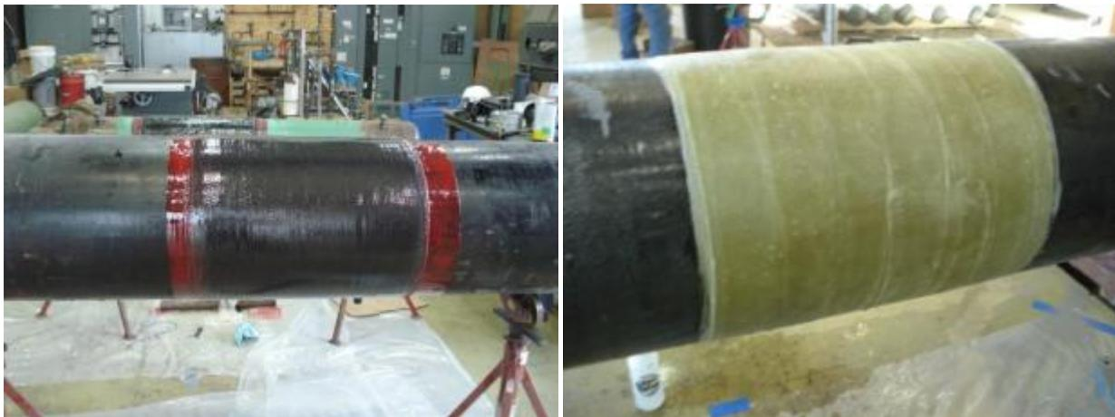
*Figure 3 - (a) Carbon fiber, (b) Glass fiber composite repairs*
