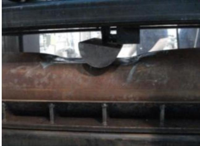
*Figure 28 - Application of dent on the pipe sample*
