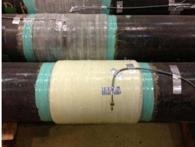
Figure 42 - View of the fiber-glass and carbon composite repairs
