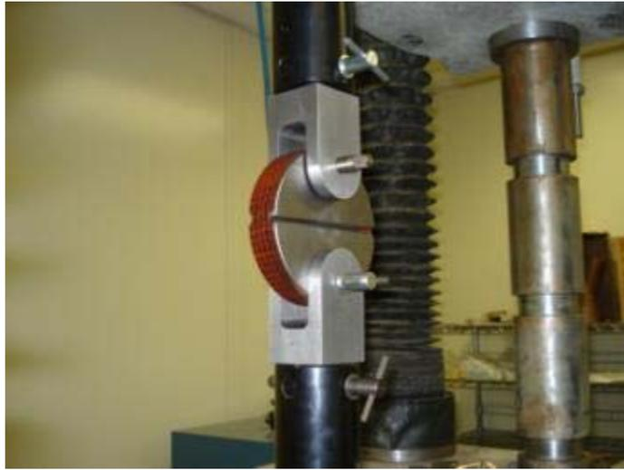
Figure 15 - ASTM D2290 tensile strength Test
