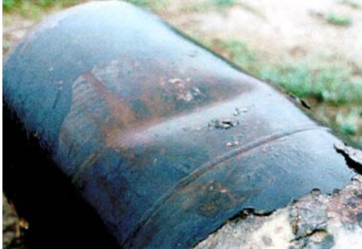
*Figure 10 - A typical dent of a large diameter pipe*
