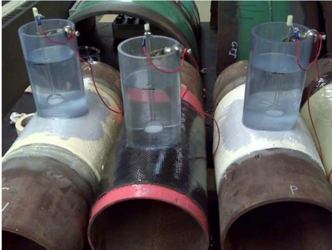
**FIGURE 7 - INSTALLATION OF THE TEST CELLS S ON THE COMPOSITE SAMPLES**
