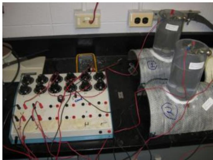
*Figure 46 - View of the cathodic disbondment testing assembly*
