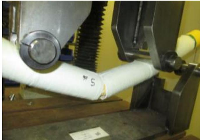
*Figure 33 - View of the composite sample after breakage in flexural test*
