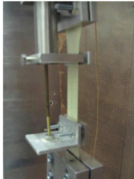
**Figures 5 & 6. Typical Fiberglass Creep Specimens**
