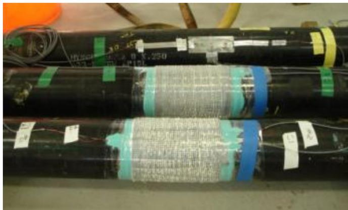
*(c) View of the control and composite-repair samples*
