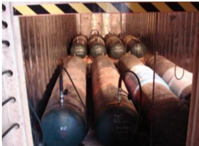
*Figure 31 - Pipe samples in the 1,000-hour pressure test*
