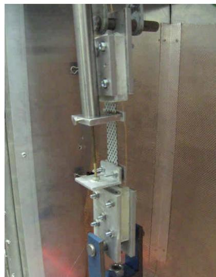
Figure 18 - Creep testing frame and sample in environmental chambers
