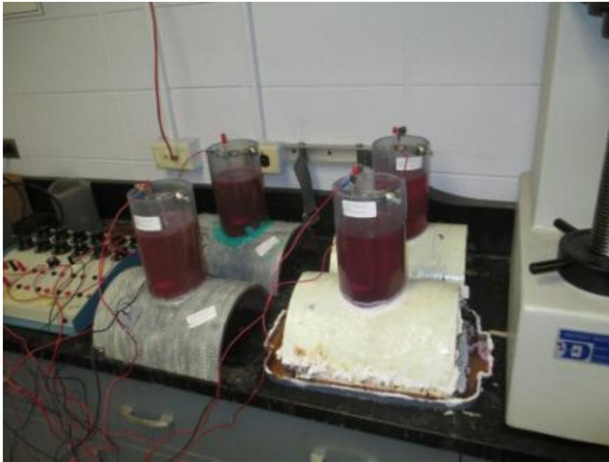
Figure 48 - View of the test assembly with dyed electrolyte
