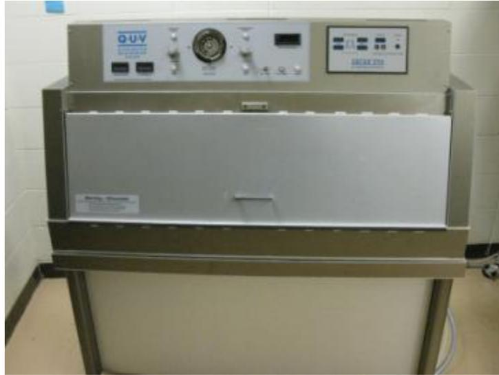
*Figure 50 - The UV light testing chamber*
