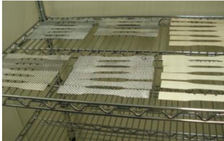
*Figure 49 - Conditioning the tensile samples for chemical exposure tests*
