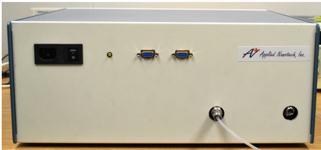
Figure 10: Front panel of GC/DMS mercaptan sensor. All connections (power, computer control, gas input) are on the front panel.
