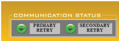
Figure 2.3 Graphical user interface tools used to report communication status between the server and the remotely located datalogger (located just off the screen in Figure 2.2).
