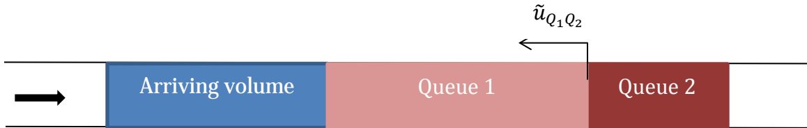
Figure E.3. Queue propagation due to capacity drop.
