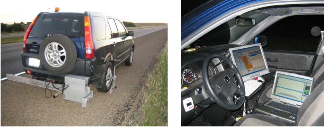
Figure 14. (a) High-speed inertial profiler mounted behind the test vehicle, and (b) test vehicle interior showing the computer screens used by the operator.
