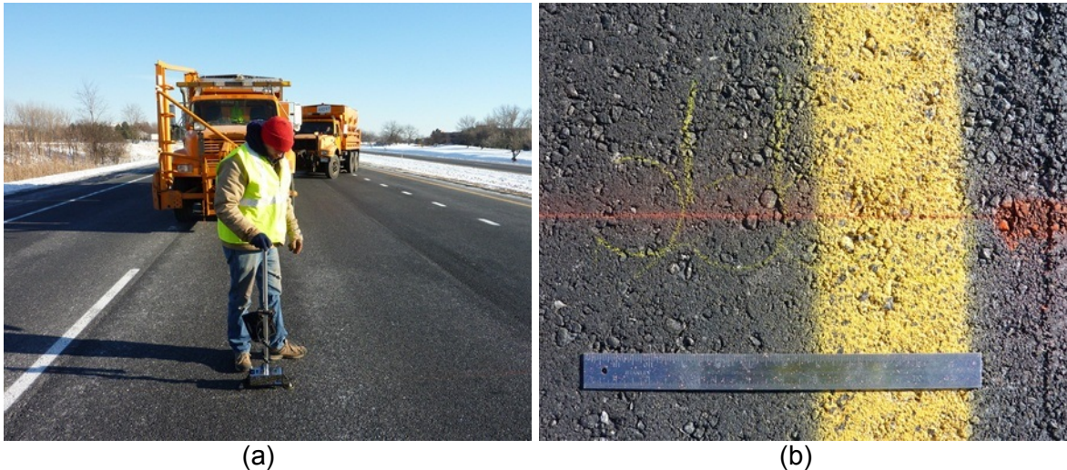
Figure 18. (a) Dipstick rut measurement, and (b) paint marking the starting point for periodical measurements.
