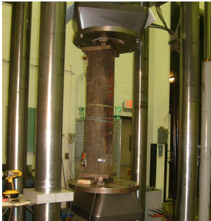
Figure 4-10. An installed specimen on the MTS testing machine.
