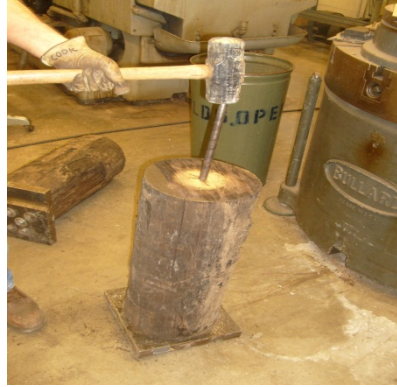
(b) Steel pin installation
