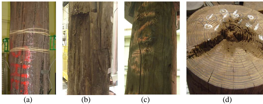
Figure 4-3. Types of decay observed in the tested pile specimens: (a) vertical crack, (b) partially crushed fibers, (c) irregular shape, and (d) mold and fungus inside of cracks.
