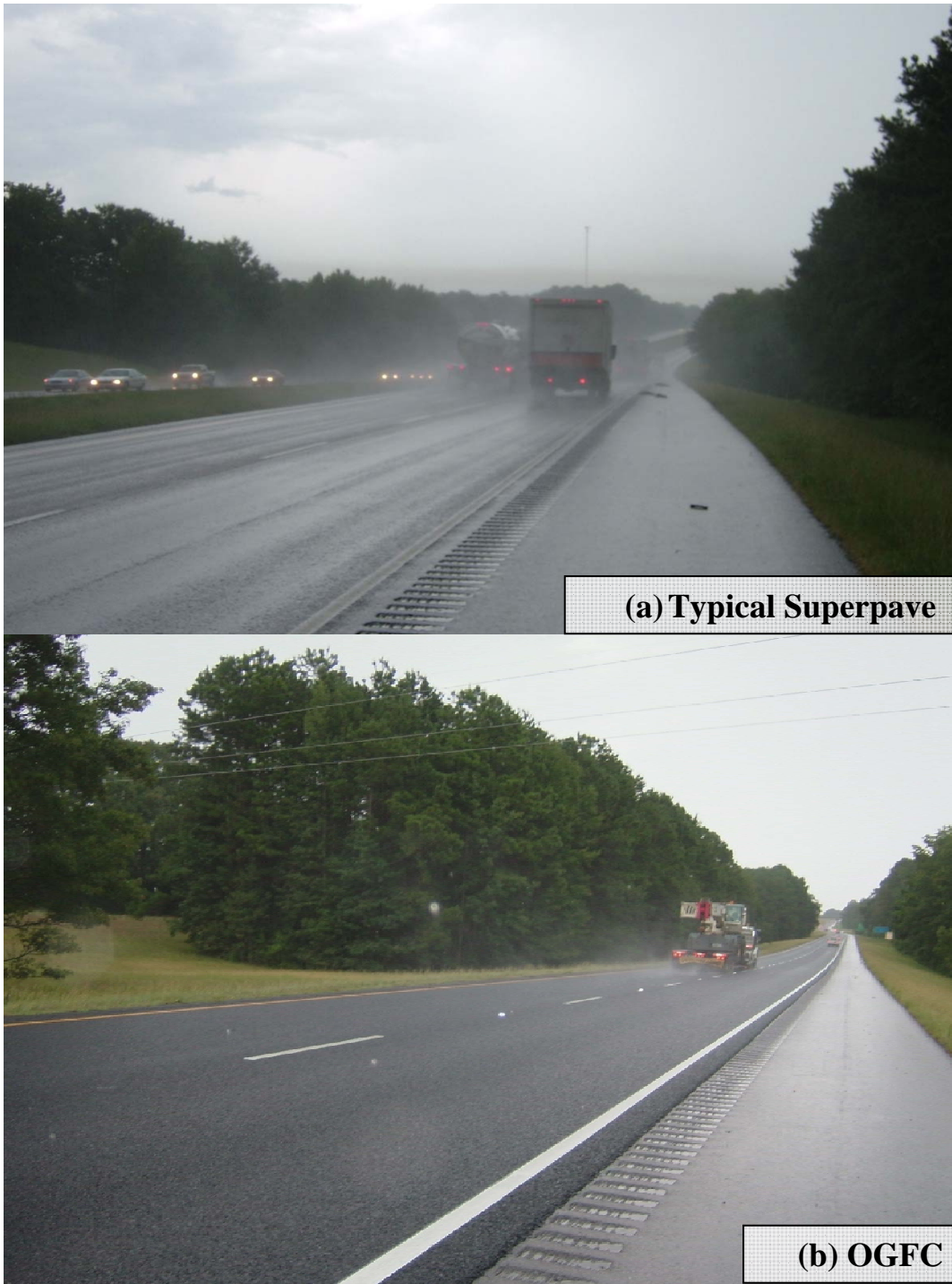
Figure 20 Splash and spray comparison: (a) typical superpave (b) OGFC
