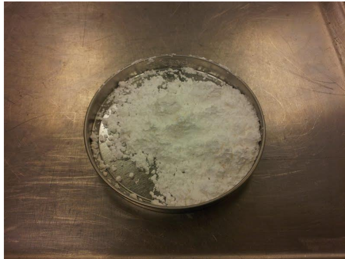
Figure 2.5 Advera synthetic zeolite WMA additive for foaming asphalt
