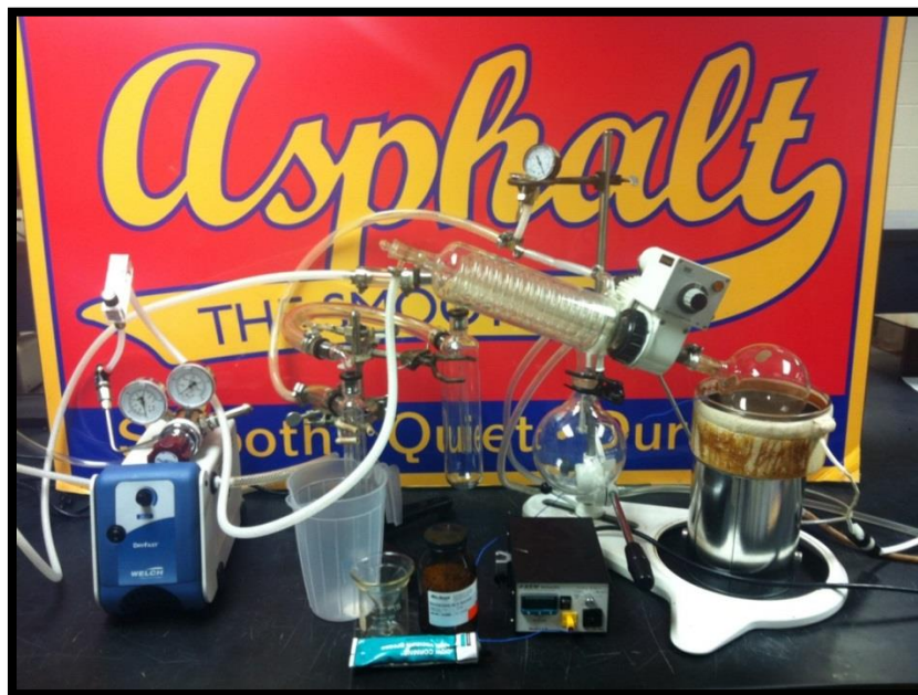
Figure 3.14 Rotavapor binder recovery system (Photo courtesy of Sheng Tang)
