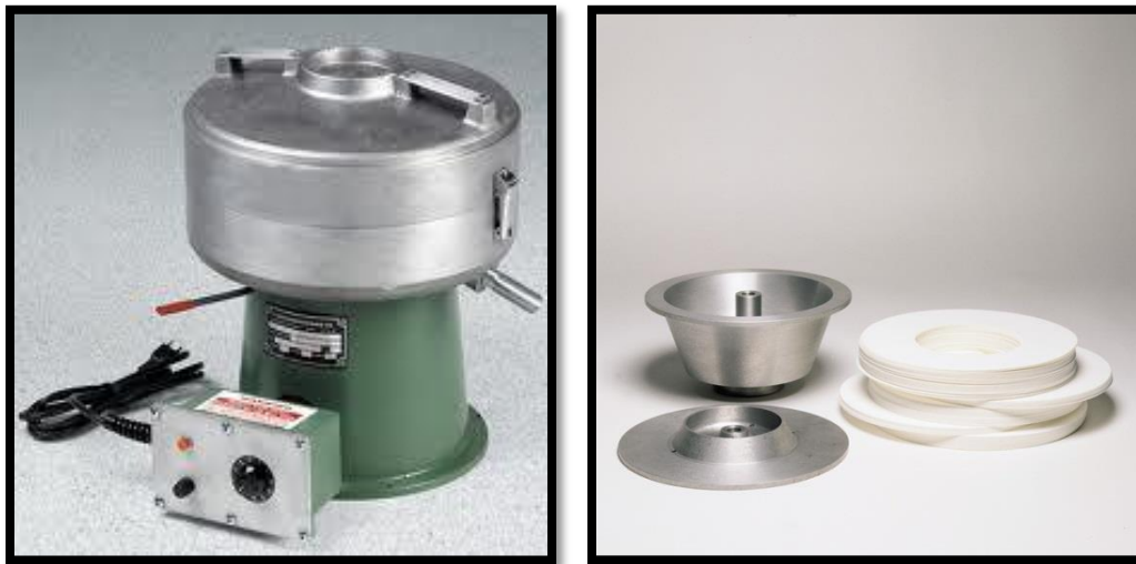
Figure 3.12 First centrifuge with bowl and filter paper
