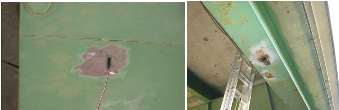
Figure 18. Weldable strain gauge
