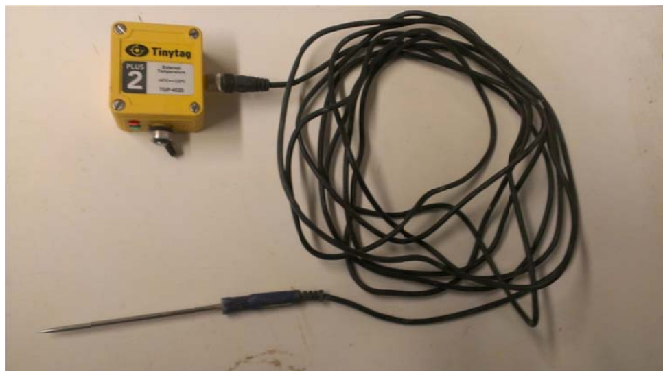
Figure 4.1: TinyTag 2.0 Temperature sensory and in-situ soil probe used for temperature measurement.
