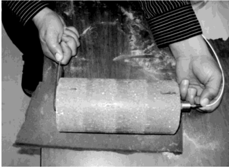
Figure 5.3: Free-free resonance testing with longitudinal excitation.
