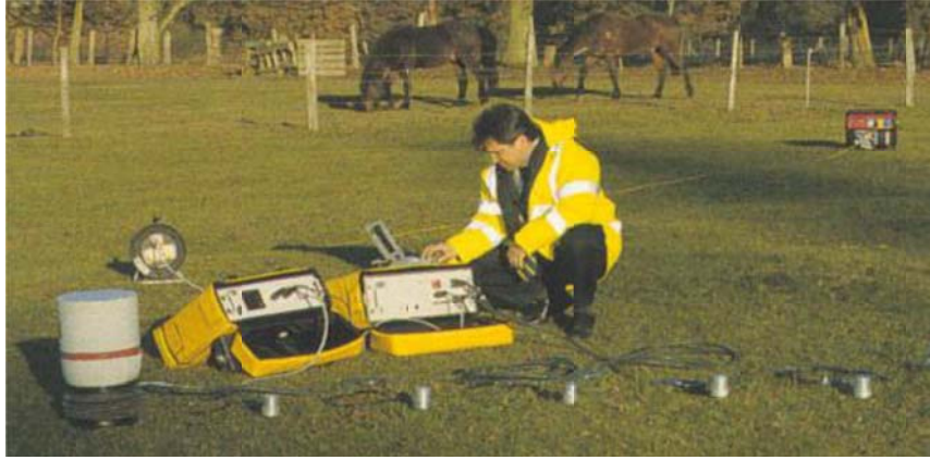
Figure 2.6: The Continuous Surface Wave System (CSWS) by GDP Instruments.
