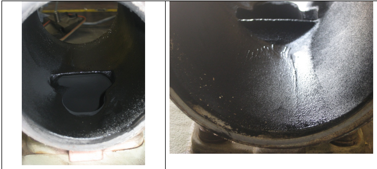
Figure 24: Interior views of power assembly cylinder showing buildup.
