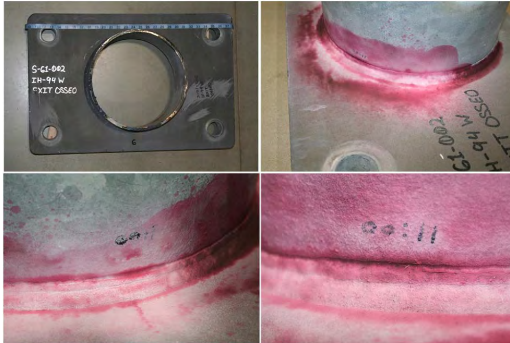
Figure 1.3 Dye Penetrant Analysis Results for S-61-002 from Osseo, Wisconsin (Diekfuss 2013).
