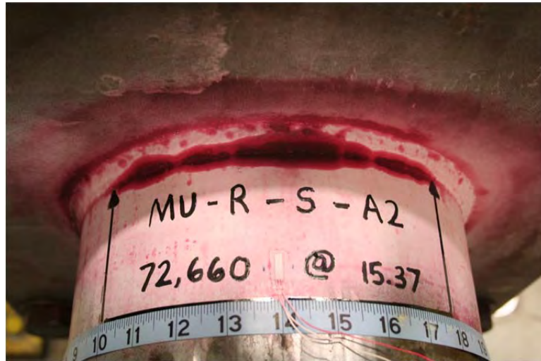
Figure 3.8 Fatigue crack detected after 72,660 cycles at 15.37 ksi on MU-CSR-R-S-A2-3.
