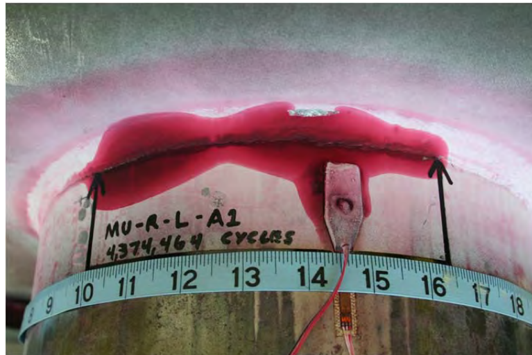
Figure 3.7 Fatigue crack detected after 4,374,464 cycles at 6.0 ksi on MU-CSR-R-L-A1-1.
