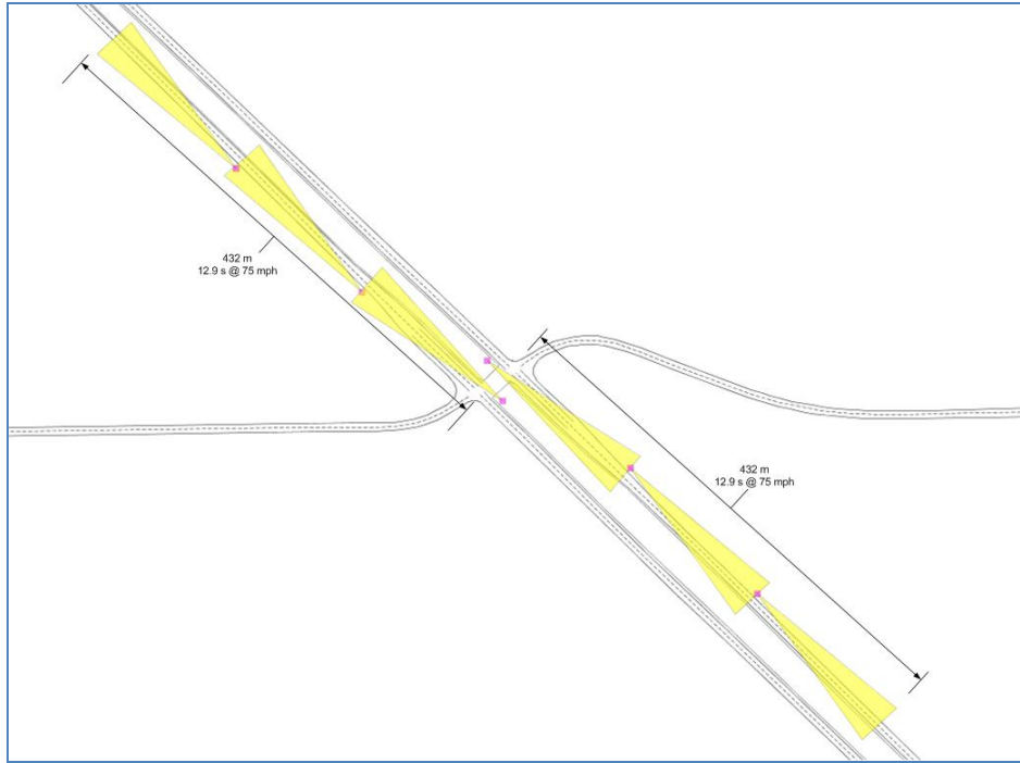
Figure 8: Minimal sensor suite layout required for mainline surveillance system on rural four lane expressway thru-stop intersections using specifications for Delphi ACC3/Eaton VS-400 radar
