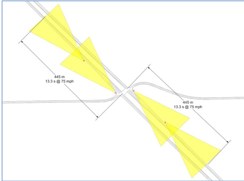
Figure 16: Minimal sensor suite layout required for mainline surveillance system on rural four lane expressway thru-stop intersections using specifications for Smartmicro UMRR
