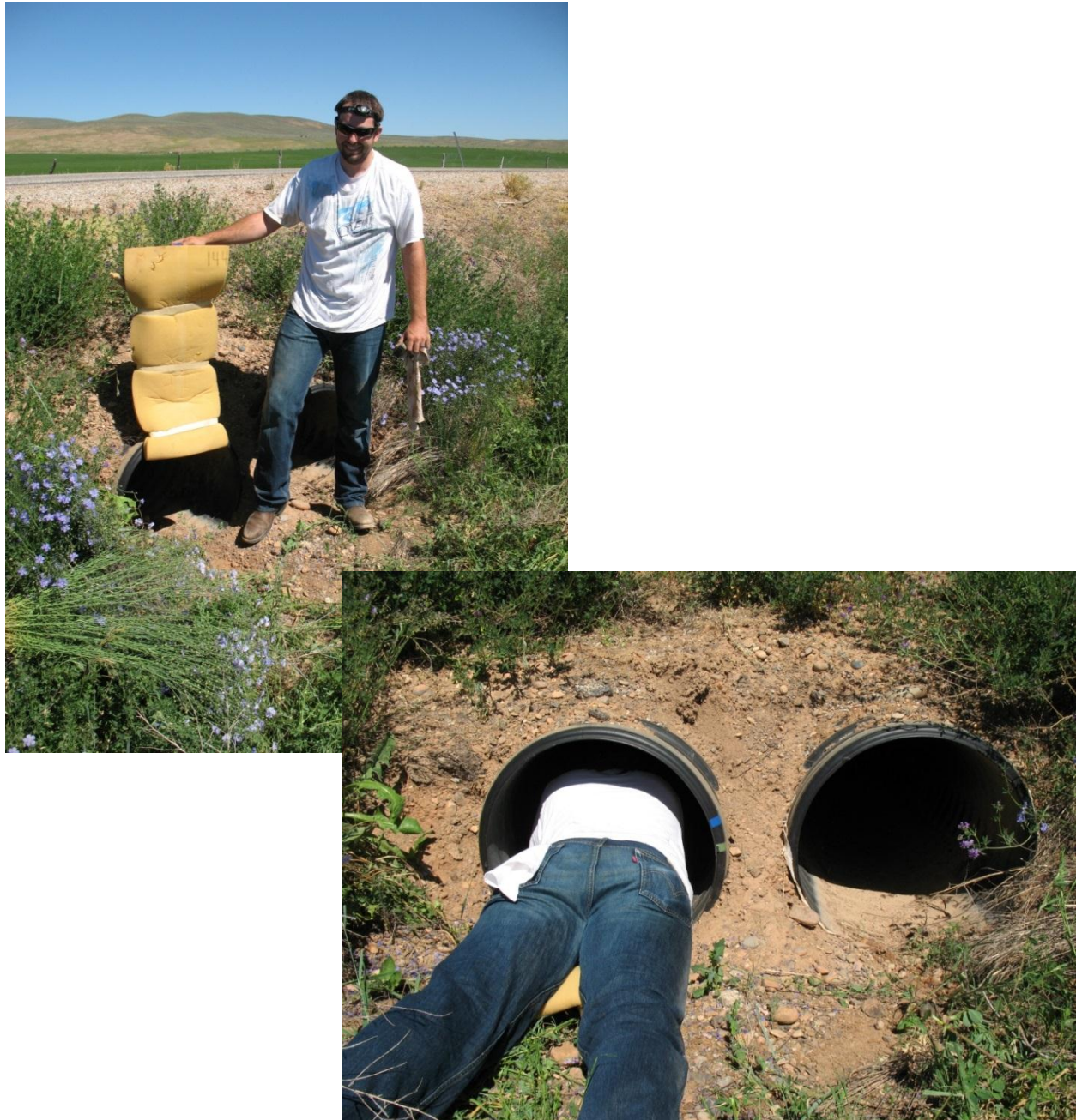
Figure 5. Photograph of the padded skate board used during pipe inspections.
