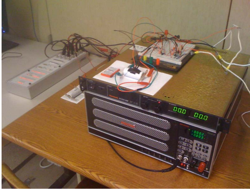
FIGURE 24 BATTERY-IN-THE-LOOP TEST BED COMPRISING A PAIR OF SORENSON POWER SUPPLY AND PROGRAMMABLE ELECTRONIC LOAD, AND A DS1103 DSPACE CONTROL BOARD.
