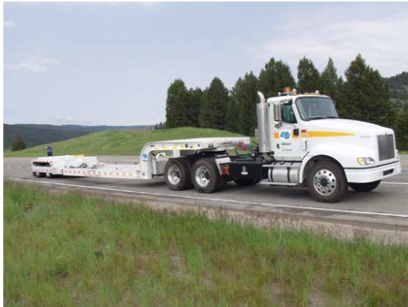
Figure 2.7: Balsi Beam Mobile Barrier ( www.dot.ca.gov )
