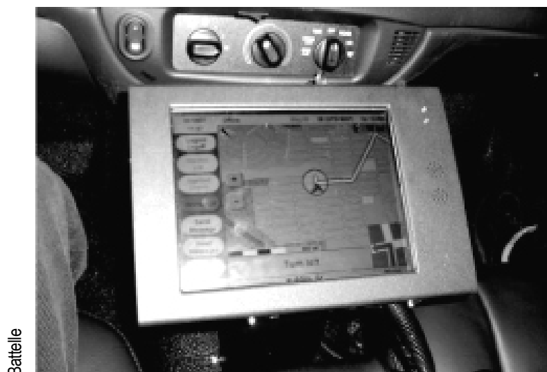
Figure 3-4. The Mobile Data Terminal is a Key In-Vehicle Information System for First Responders
