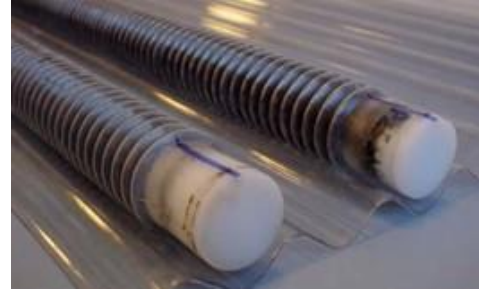
(b) line mark on the corrugated tubes
