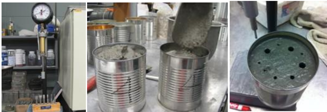
Figure 3.5. Test photos for final set time of mortar
