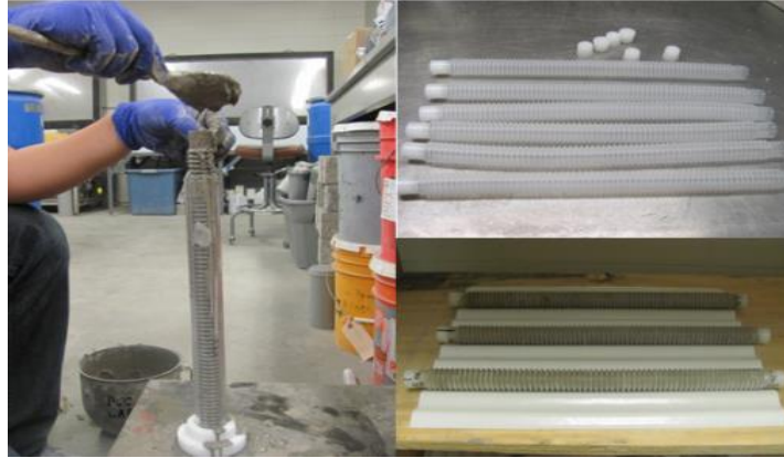
Figure 3.4. Specimen preparations for autogenous shrinkage of mortar
