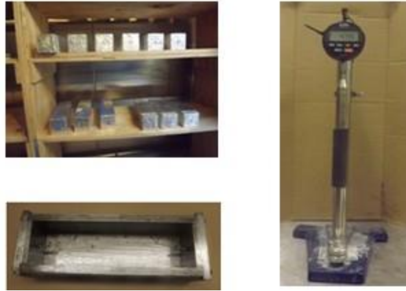
Figure 3.7. Samples, molds, and comparator for concrete autogenous shrinkage measurement
