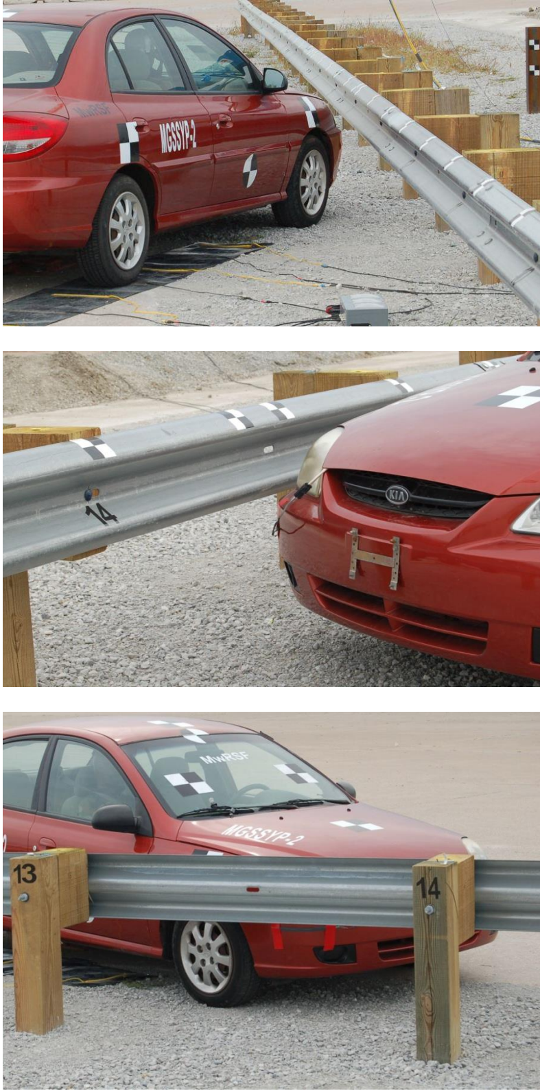
Figure 52. Impact Location, Test No. MGSSYP-2
