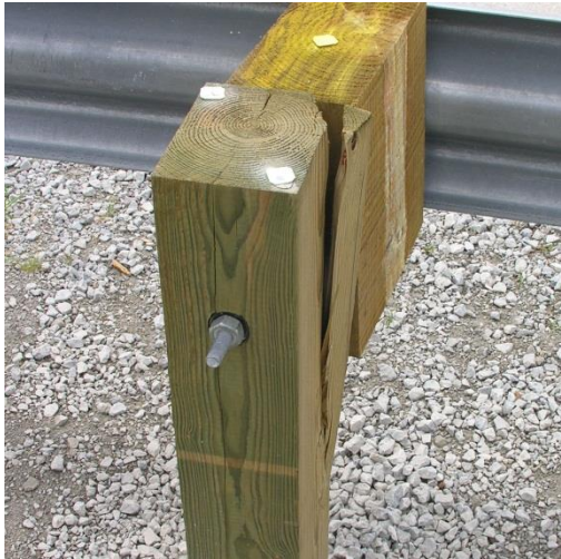
Figure 39. Post Nos. 6 and 10 Damage, Test No. MGSSYP-1
