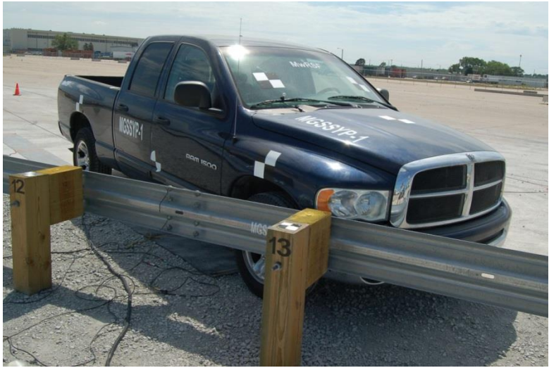
Figure 35. Impact Location, Test No. MGSSYP-1
