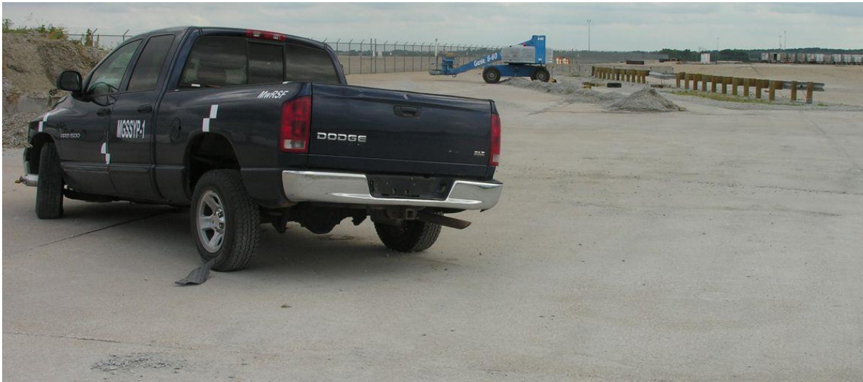
Figure 36. Vehicle Final Position and Trajectory Marks, Test No. MGSSYP-1
