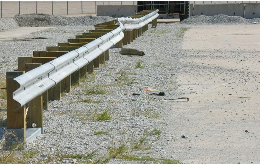
Figure 54. System Damage, Test No. MGSSYP-2
