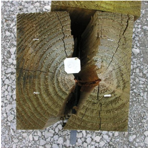
Figure 40. Post Nos. 11 and 12 Damage, Test No. MGSSYP-1.
