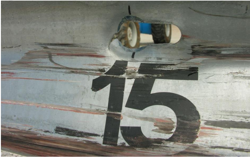
Figure 55. Rail Damage Between Post Nos. 13 and 15, Test No. MGSSYP-2
