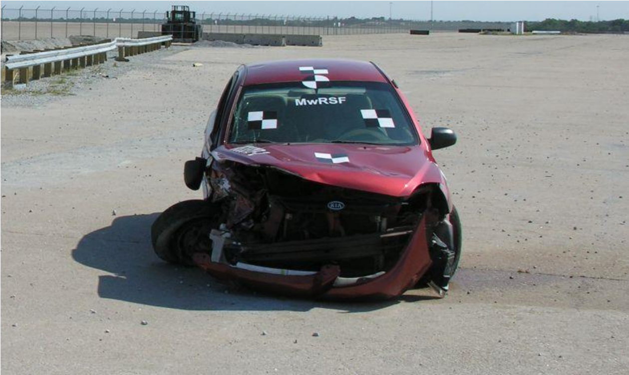
Figure 53. Vehicle Final Position and Trajectory Marks, Test No. MGSSYP-2
