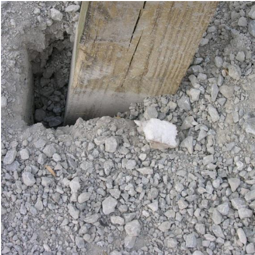
Figure 59. Post Nos. 17 and 18 Damage, Test No. MGSSYP-2
