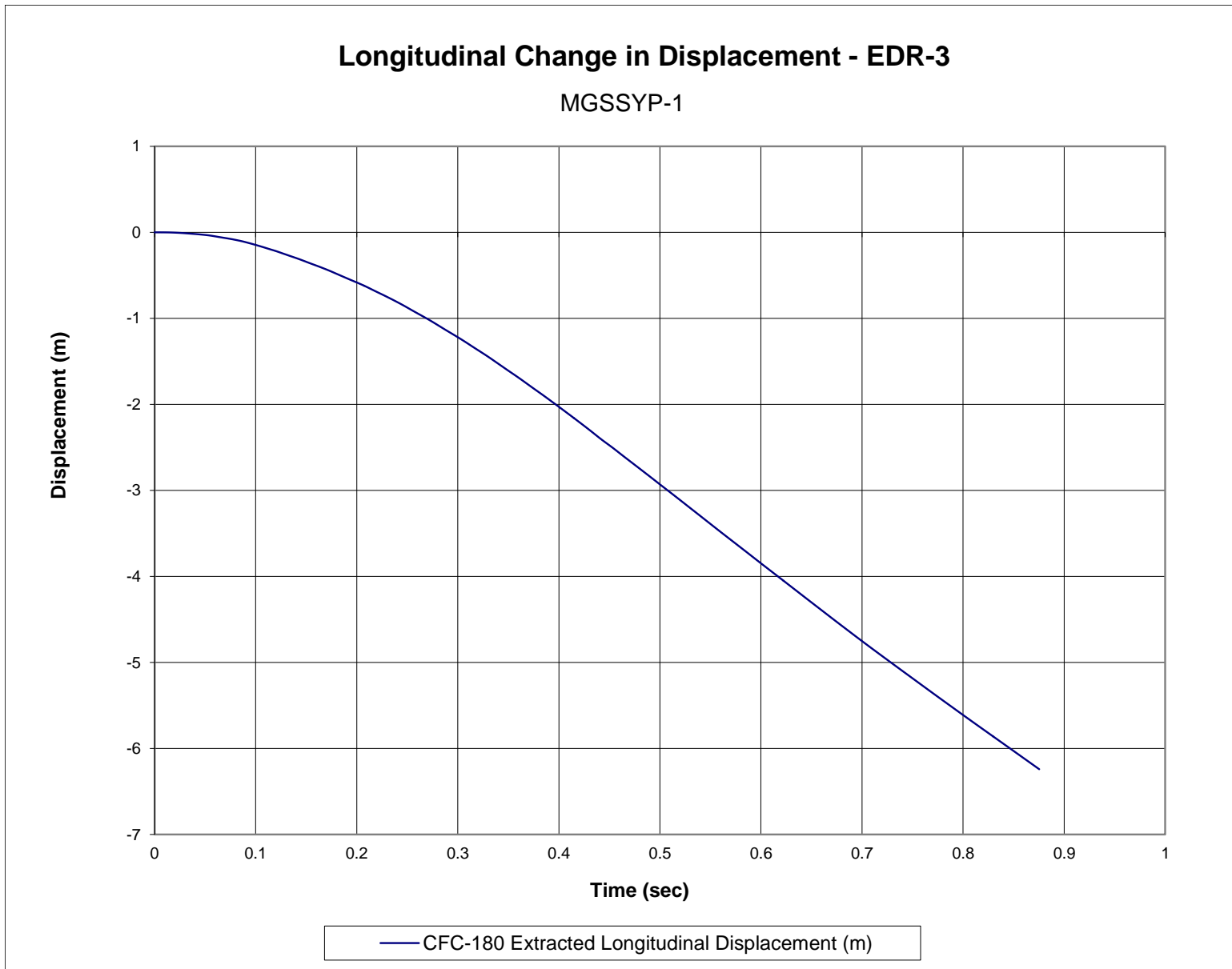
Figure E-11. Longitudinal Occupant Displacement (EDR-3), Test No. MGSSYP-1
