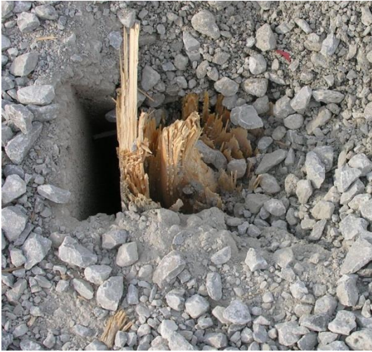
Figure 58. Post Nos. 15 and 16 Damage, Test No. MGSSYP-2
