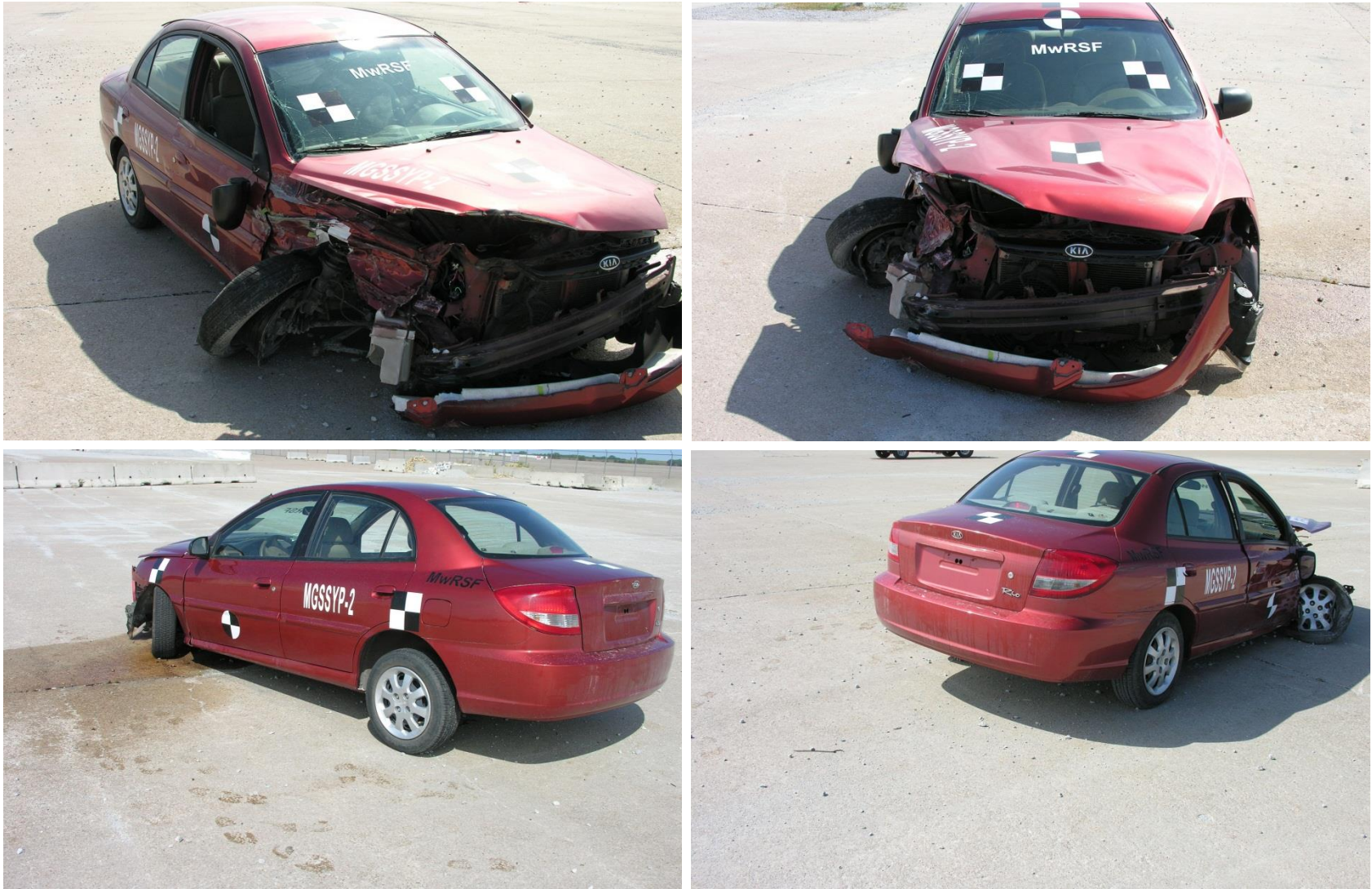
Figure 61. Vehicle Damage, Test No. MGSSYP-2
