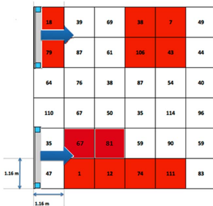
Figure 91. Spatial distribution of k-values with axle loading on RE and LE for option selected for Case R-36 Option IV.
