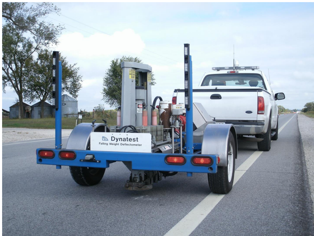
Dynatest 8000 Falling Weight Deflectometer Tester
