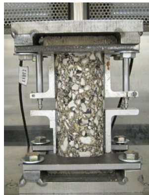
FIGURE 3.6 Direct Testing Fatigue Test Set Up
