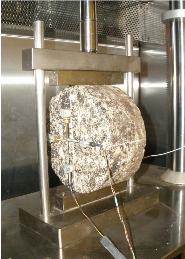
FIGURE 3.5 AASHTO TP-9 Setup
