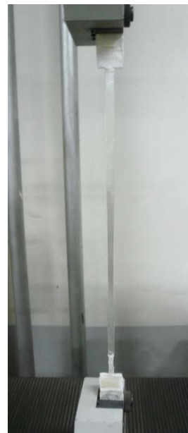
Figure 12 Tensile Tests of Non-Impregnated and Impregnated Fiber Rovings (Choi et al. [24]) (a) Tensile testing of bare CF roving (b) Tensile testing of impregnated GF roving
