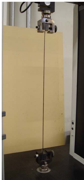
Figure 12 Tensile Tests of Non-Impregnated and Impregnated Fiber Rovings (Choi et al. [24]) (a) Tensile testing of bare CF roving (b) Tensile testing of impregnated GF roving
