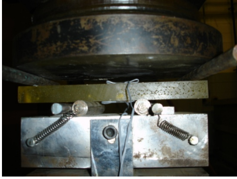
Figure 11 Four-Point Loading Tests of J and K Type Epoxy Resin Blocks (Choi et al. [24]; Song et al. [25]) (a) Bending testing of J type epoxy resin block (b) Bending testing of K type epoxy resin block
