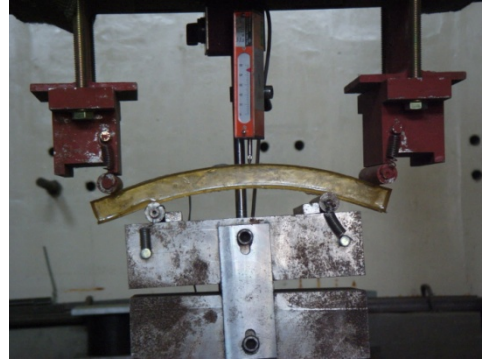
Figure 11 Four-Point Loading Tests of J and K Type Epoxy Resin Blocks (Choi et al. [24]; Song et al. [25]) (a) Bending testing of J type epoxy resin block (b) Bending testing of K type epoxy resin block
