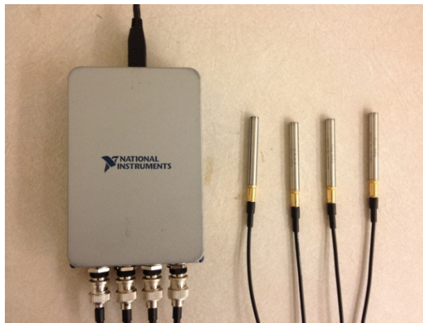
Figure 5.16 a NI cDAQ 9171 USB chassis and four microphones
