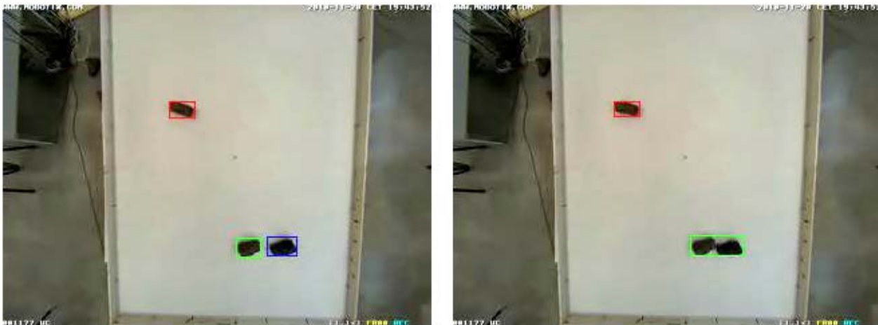
Figure 4.18 Illustration of accident detection by identifying the change in area that occurs when two vehicles are detected as a single, combined vehicle
