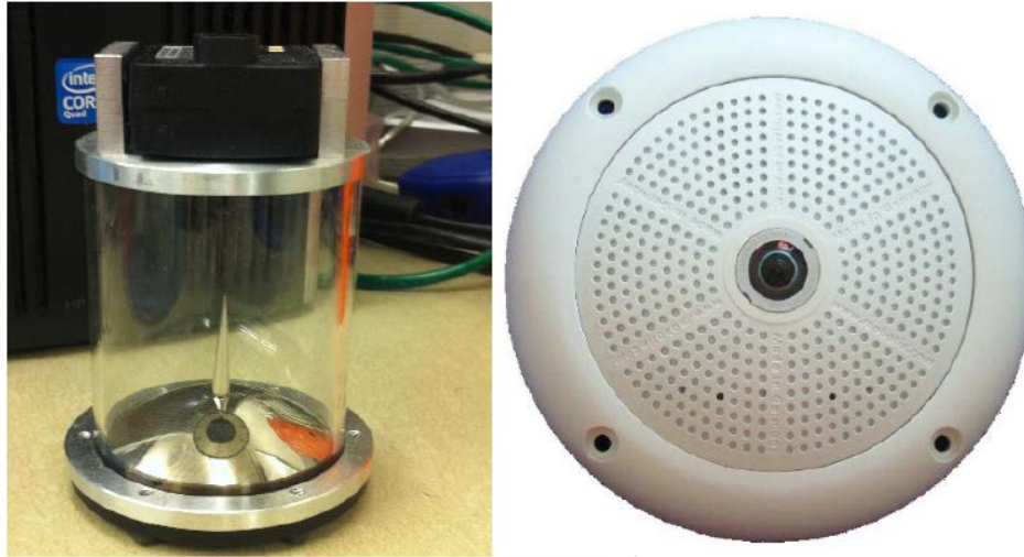
Figure 3.2 The catadioptric camera (left) and the fish-eye camera (right)
