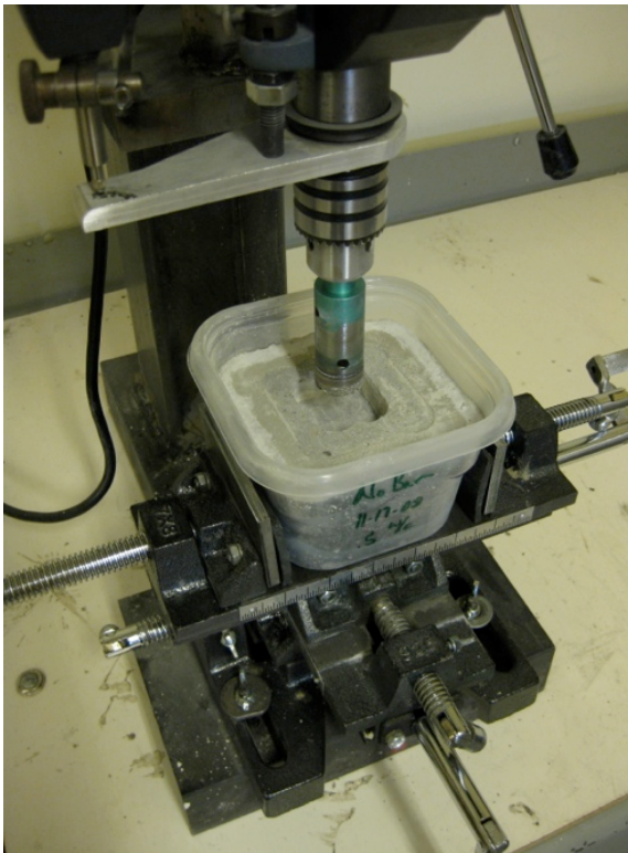
Figure 7: A powder sample being collected from a concrete sample after being exposed to a sodium chloride solution for a given time.
