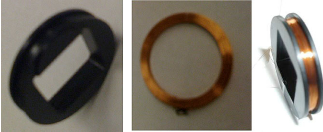
Figure 12a: New RFID sensor body, prototype coil and sensor body and coil.
