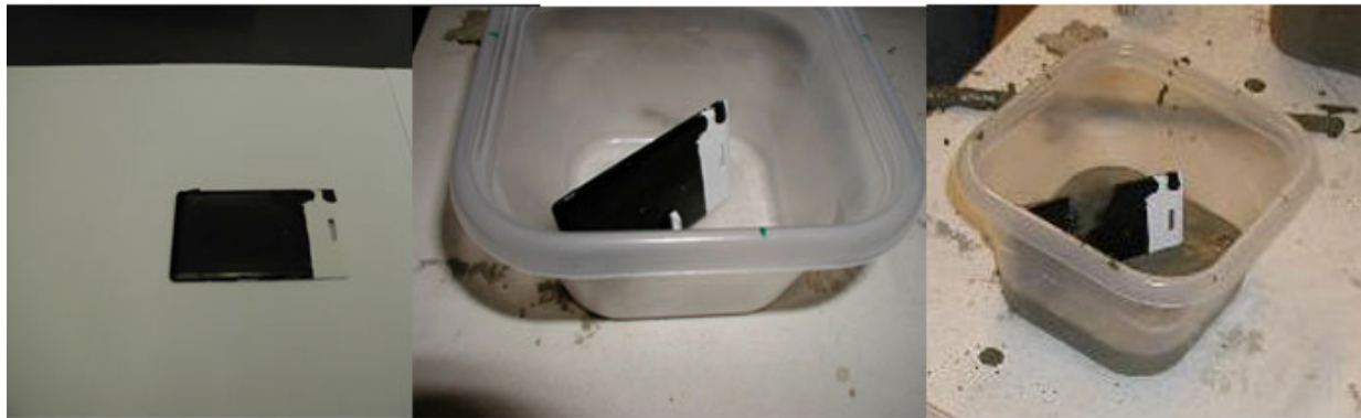
Figure 10: Larger RFID based corrosion sensor being embedded in concert for accelerated corrosion testing.
