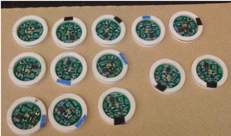
Figure 17a: Sensors after the coils have been wound and attached to the electronics.
