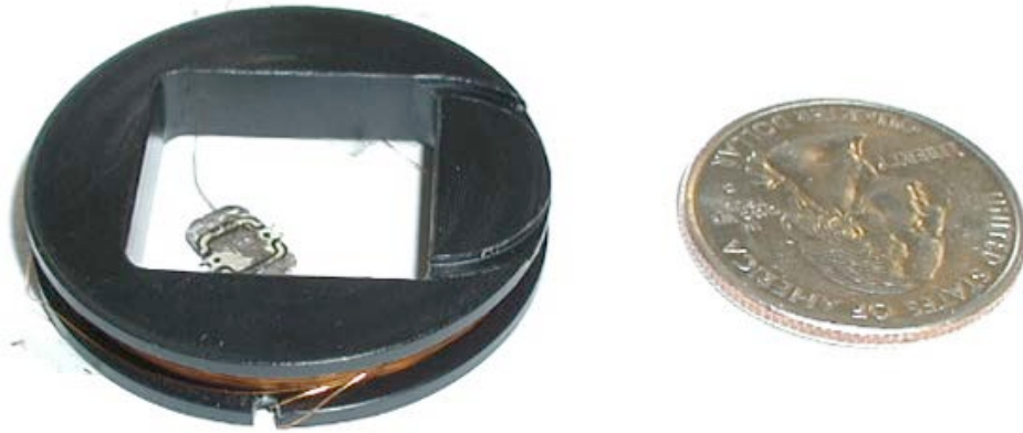
Figure 13: New RFID sensor with a commercial RFID chip and a quarter for size reference.
