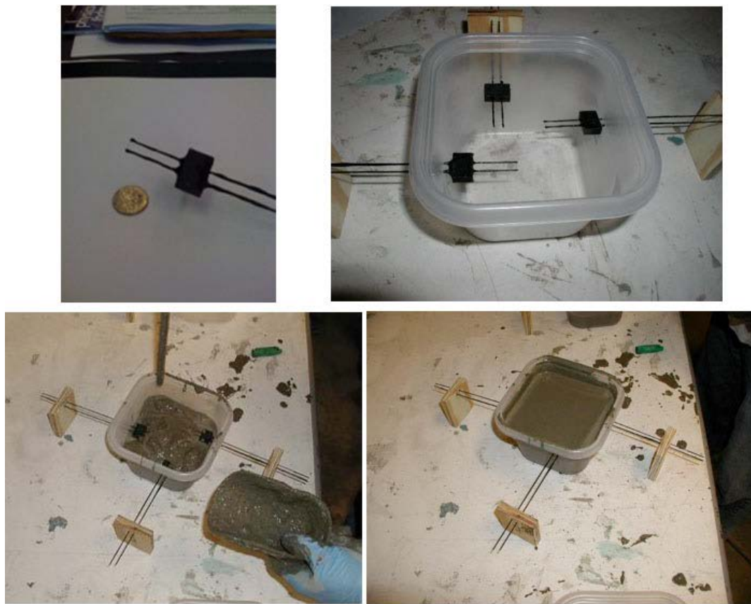
Figure 9: The wire holder for testing our triggering system is shown on the top left. The next pictures show three of these holders being embedded in concrete for accelerated corrosion testing.
