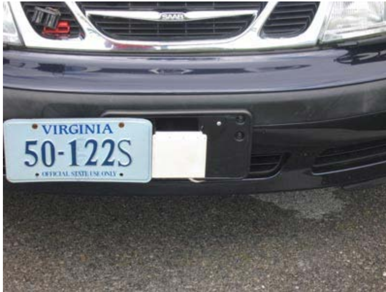
Figure 3: Placement of radar on front license plate frame (SHRP2, 2010)
