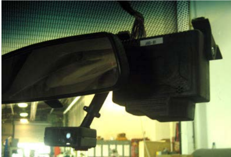
Figure 1: Mounting of the head unit in an instrumented vehicle (SHRP2, 2010)
