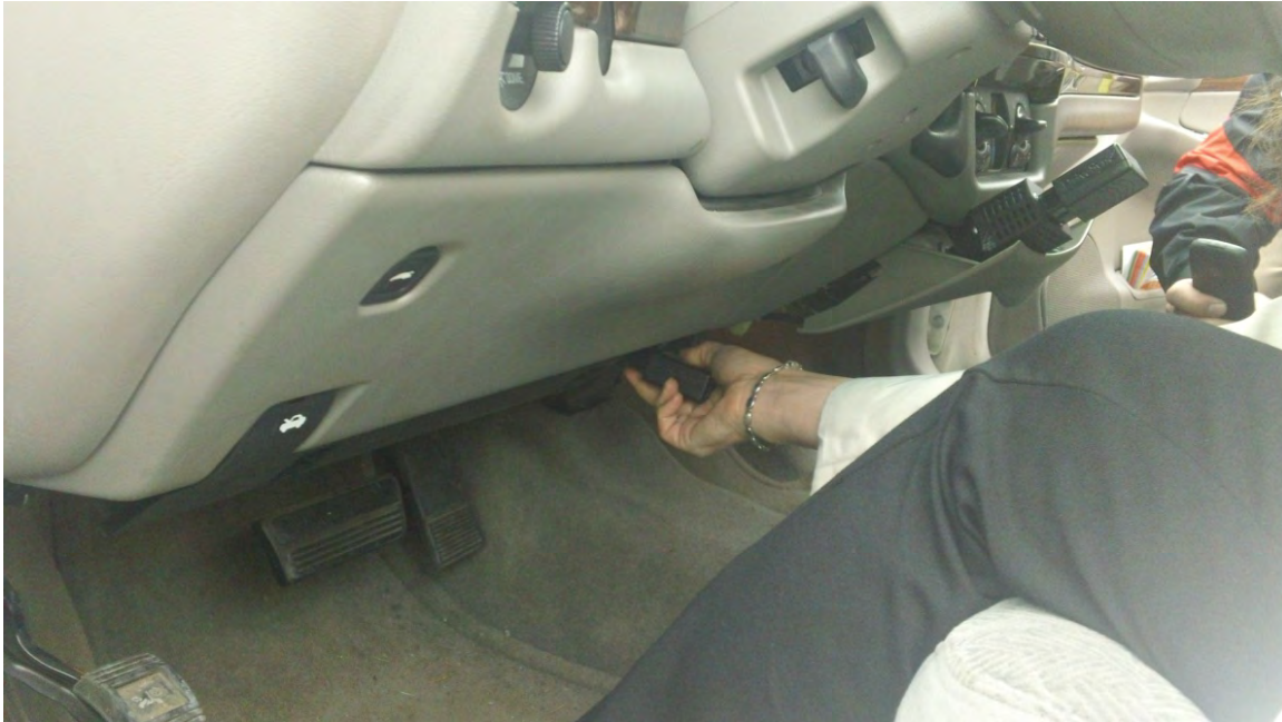
Figure 3: Typical Installation of Mileage Reporting Device
