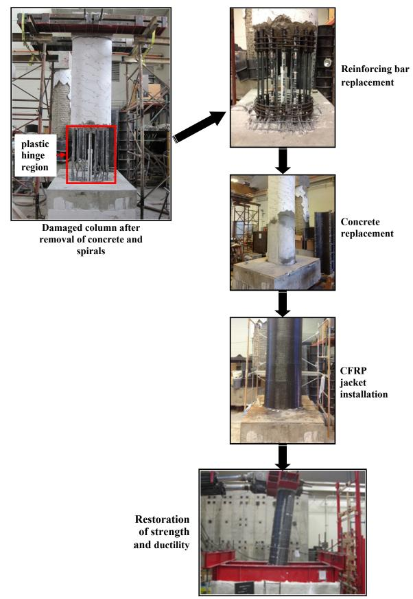
Figure 1: Repair of column with interlocking spirals and fractured longitudinal bars
