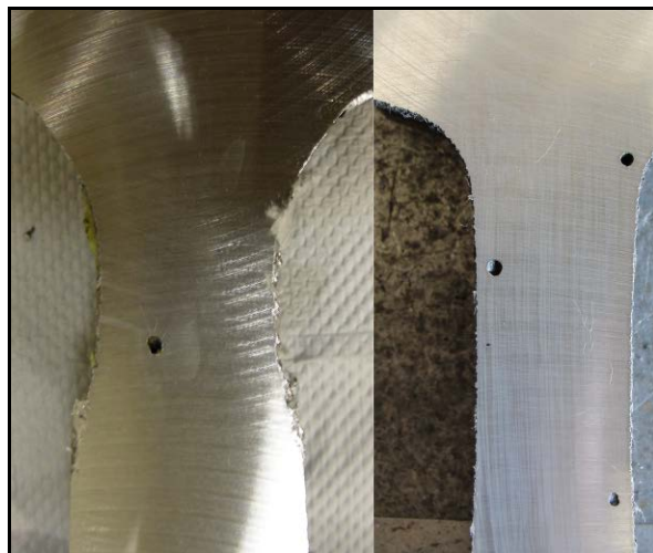
Figure 4. Gas Holes in Railtech Welds R4 (left) and R12 (right)
