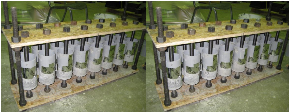
Figure 3.4. Direct tension test UHPC half-specimen jig
