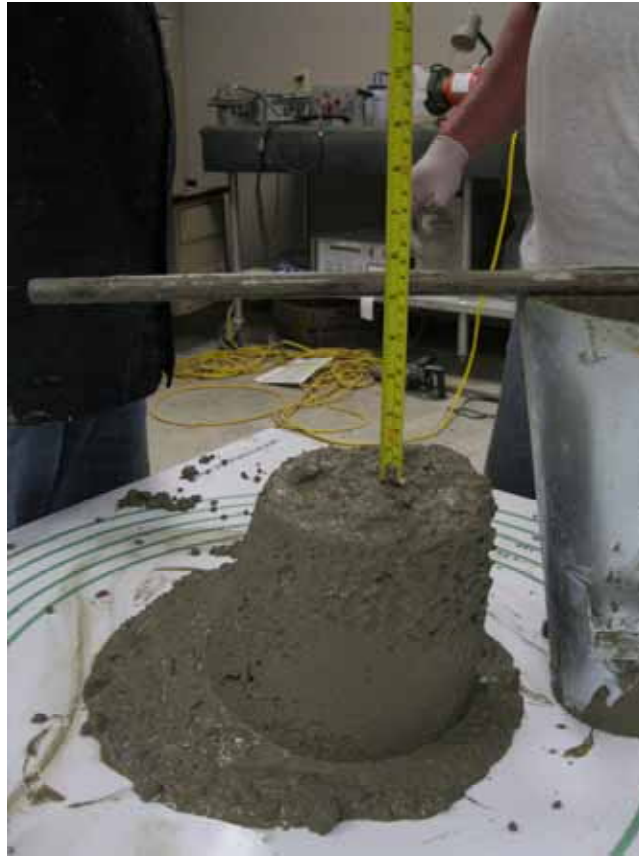
Figure 22 - Post-Vibrated Slump and Base Spread
