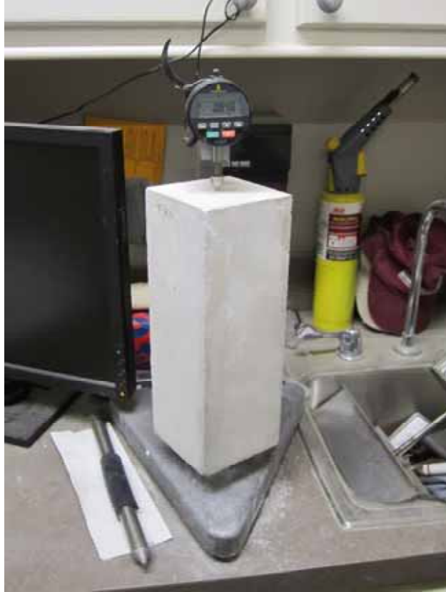
Figure 24 - Comparator Reading of Concrete Specimen
