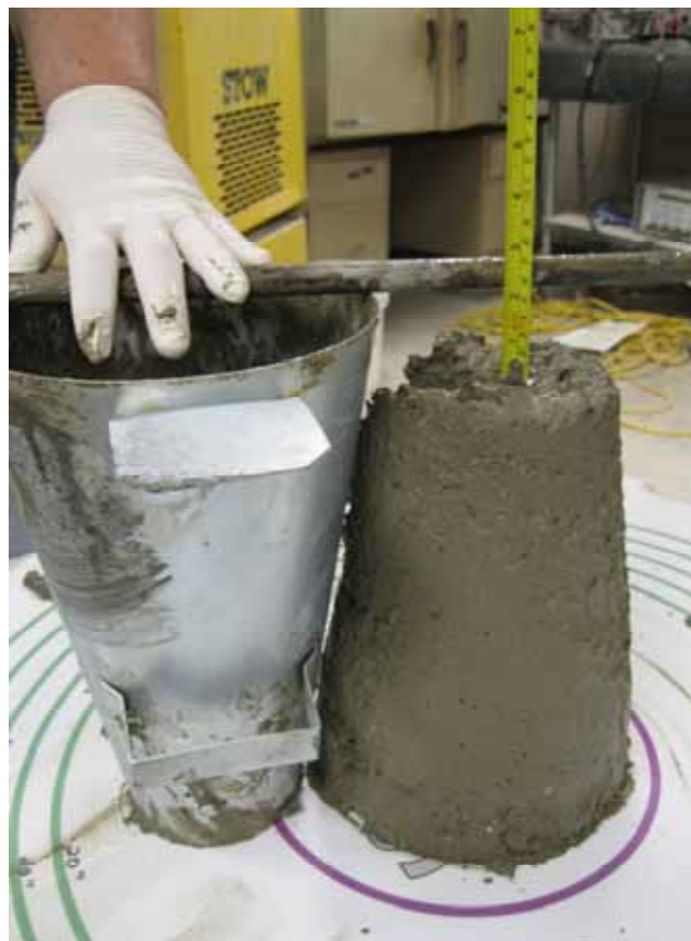
Figure 21 - Pre-Vibrated Slump and Base Spread
