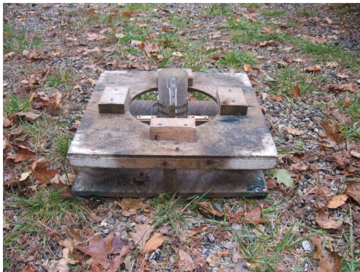
Figure 8: Surface Inundation Test Equipment; A variation on ASTM C 1701 and D 3385-03
