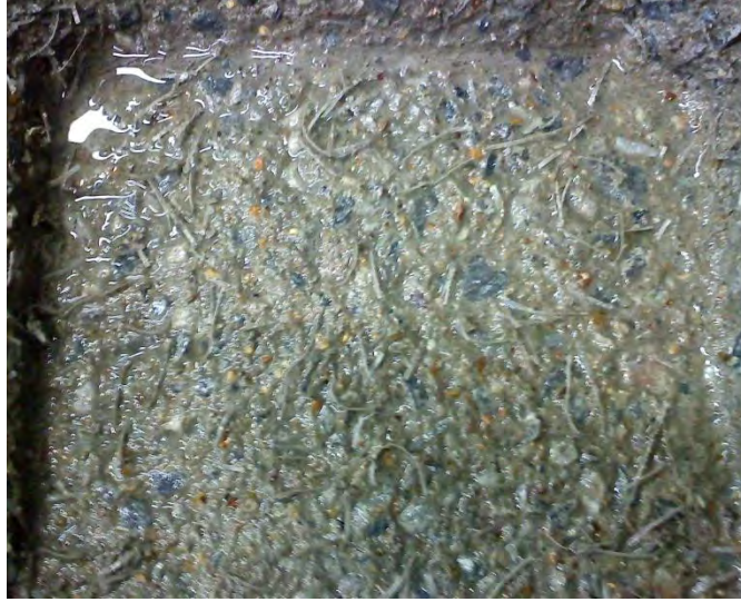
Figure 21. New Hampshire salt scaling sample after 50th freeze-thaw cycle
