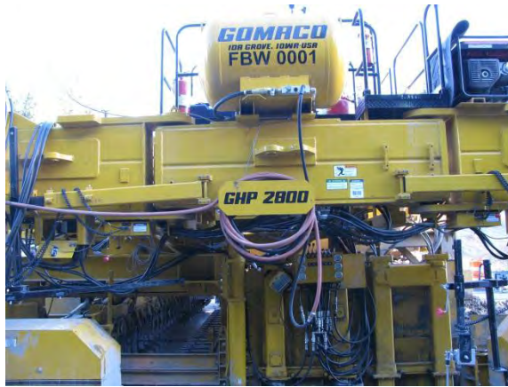
Figure 9. GOMACO GHP 2800 slipform concrete paver
