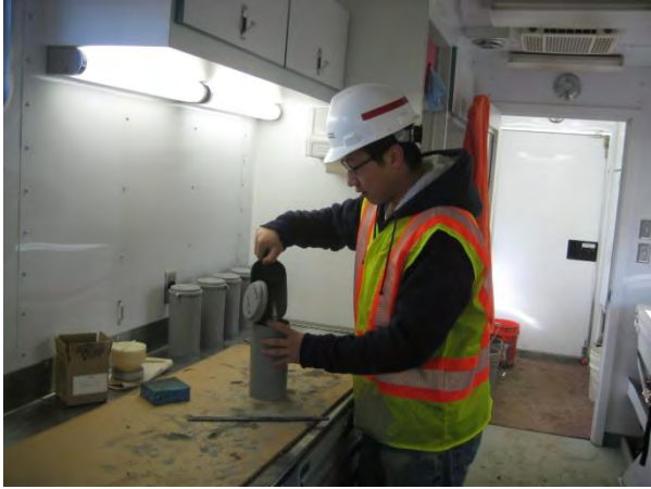
Figure 8. Preparing concrete cylinder samples
