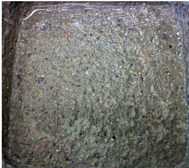
Figure 23. PA salt scaling sample after 50th freeze-thaw cycle
