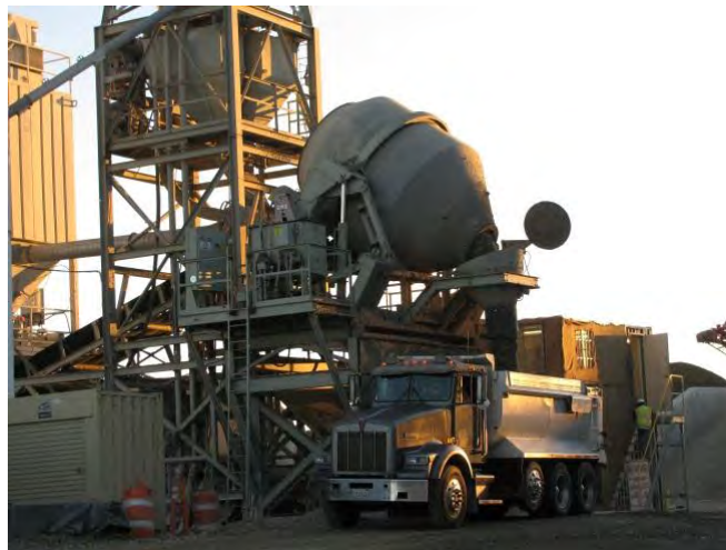
Figure 6. Concrete being discharged at central mix plant
