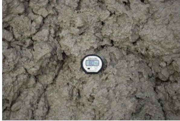
Figure 13. Concrete temperature being tested by sensor
