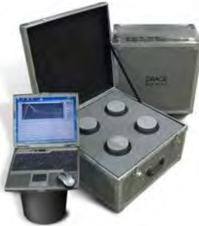
Figure 15. Adiacal calorimetry test equipment for heat of hydration of concrete
