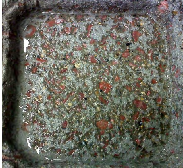
Figure 18. IA salt scaling sample after 50th freeze-thaw cycle
